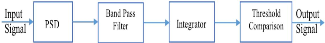
**Figure 2.12: Energy detector block diagram.**
