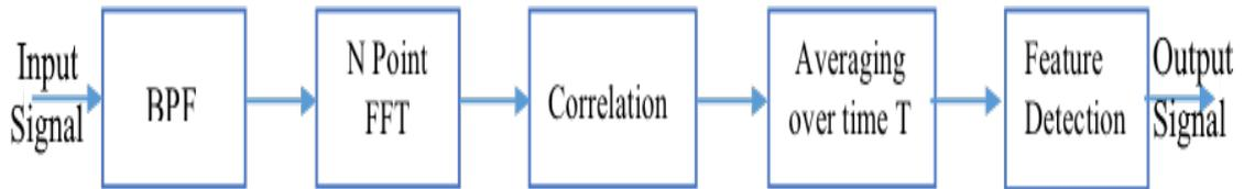
**Figure 2.13: Block diagram for cyclostationary feature detection.**
