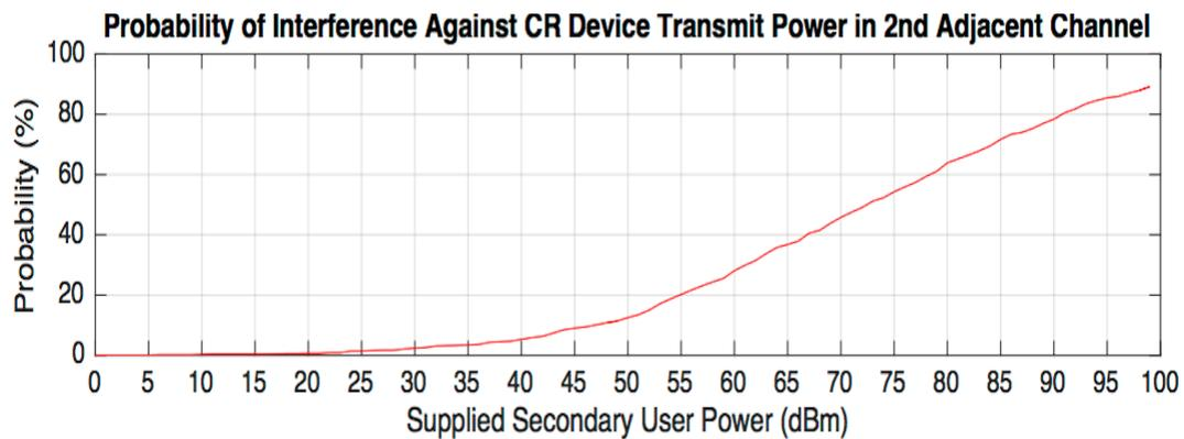
**Figure 3.7: Probability of interference against transmit power of 2<sup>nd</sup> Adjacent SU.**
