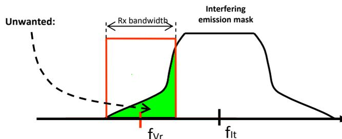
**Figure 2.4: Interference due to the unwanted emissions.**
