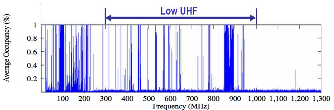
**Figure 2.1: Spectrum Occupancy Measurements.**
