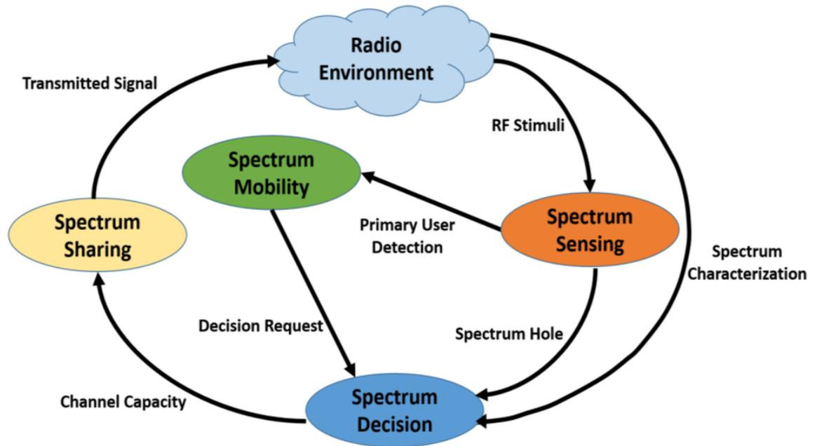
**Figure 2.9: The cognitive cycle in detecting spectrum holes.**
