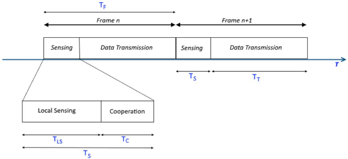
**Figure 4.5: Communication frame for secondary cognitive radio networks.**
