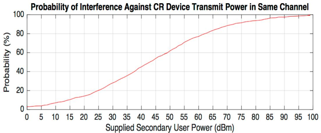
**Figure 3.3: Probability of interference against transmit power of co-channel SU.**
