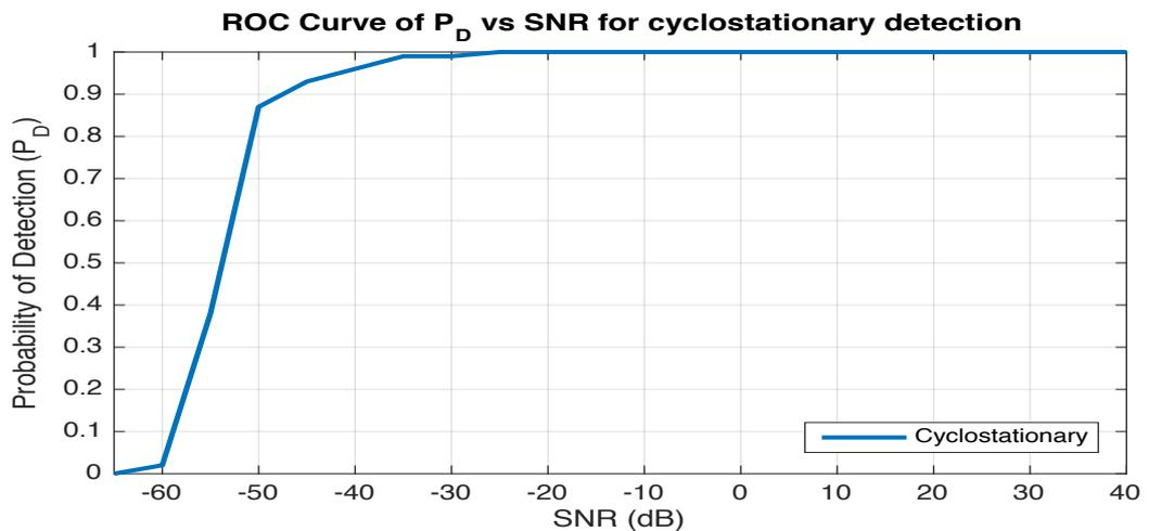
**Figure: 5.5: Cyclostationary detector performance.**
