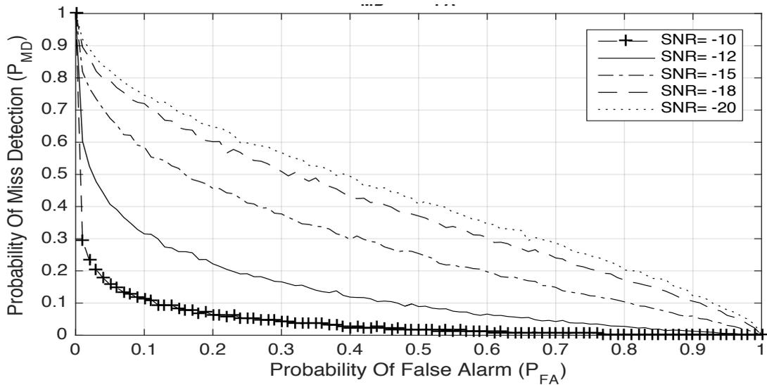
**Figure 3.10: Energy Detection ROC curve for  $P_{MD}$  vs  $P_{FA}$  with varying SNR.**
