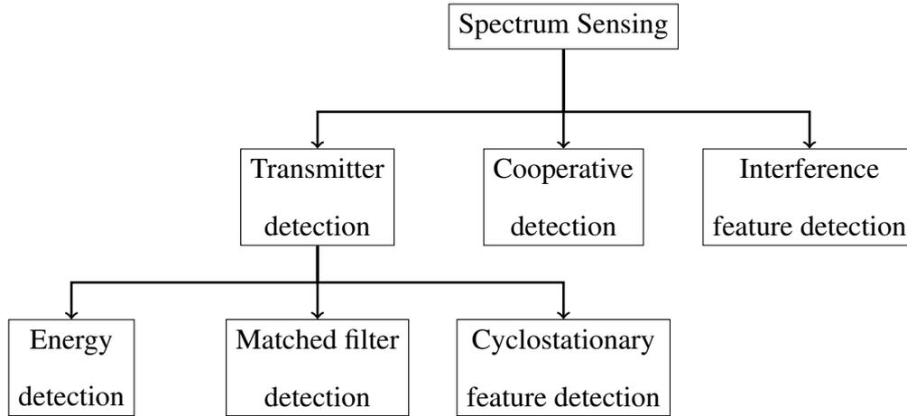
**Figure 2.10: Classification of spectrum sensing techniques.**
