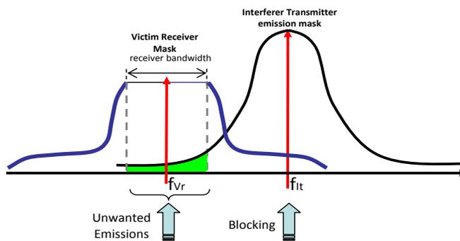
**Figure 2.6: Combined unwanted emissions and receiver blocking mechanism.**
