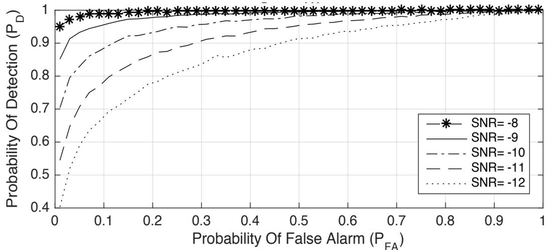
**Figure 3.9: Energy Detection ROC curve for  $P_D$  vs  $P_{FA}$  with varying SNR.**
