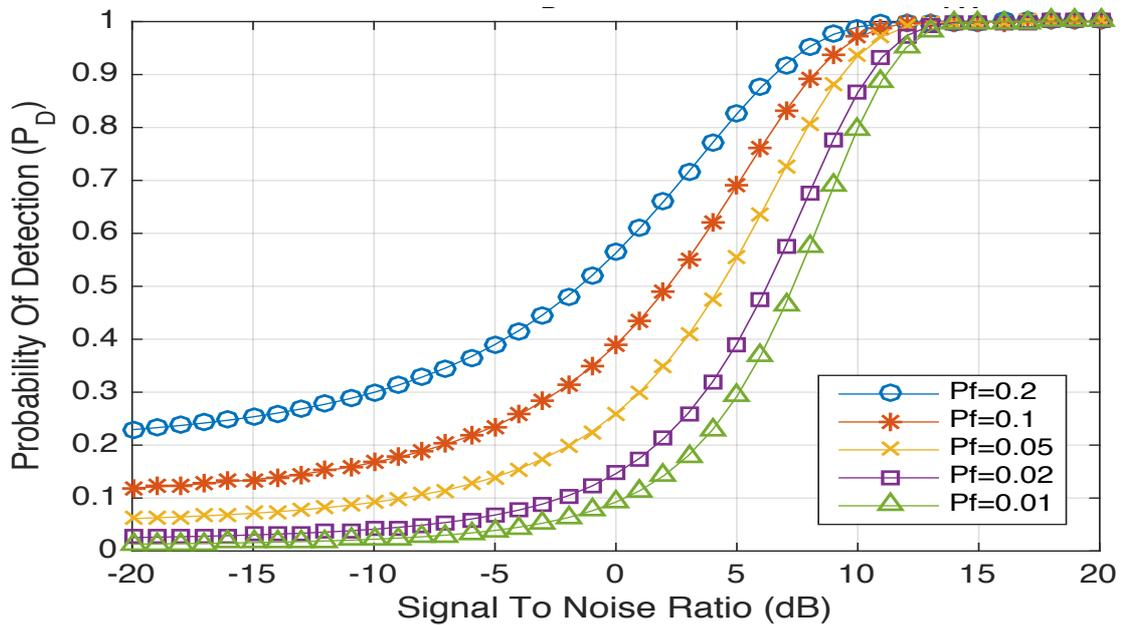
**Figure 3.11: Matched Filter Detection ROC curve for  $P_D$  vs SNR.**
