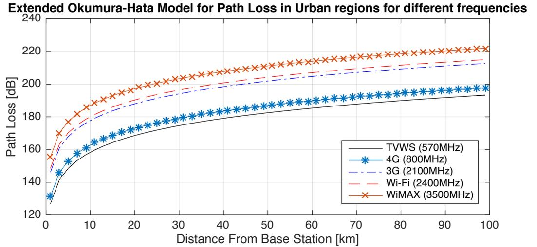
**Figure 5.1: Extended Okumura-Hata Path loss Comparison.**
