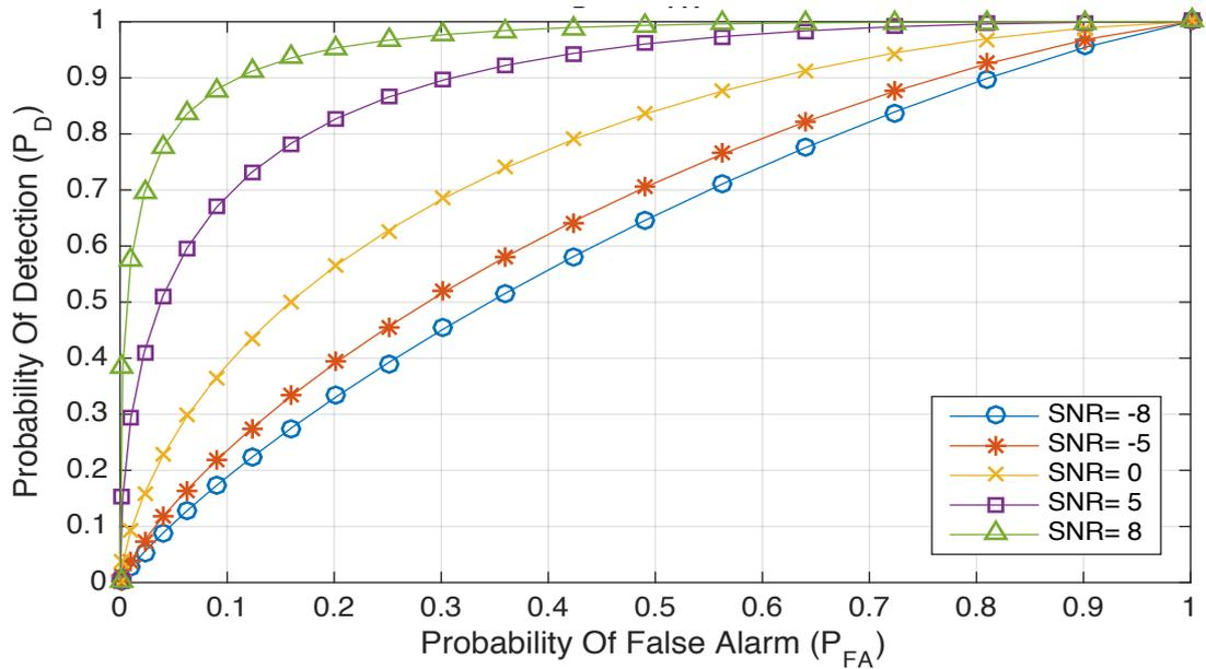
**Figure 3.12: Matched Filter Detection ROC curve for  $P_D$  vs  $P_{FA}$ .**
