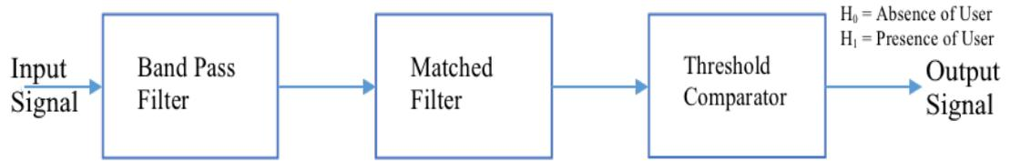
**Figure 2.11: Block Diagram for Matched Filter Detection.**
