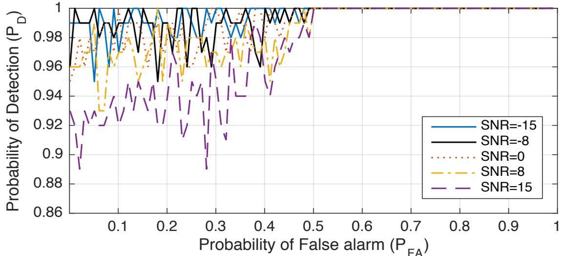
**Figure 3.14: Cyclostationary Detection ROC curve for  $P_D$  vs  $P_{FA}$ .**
