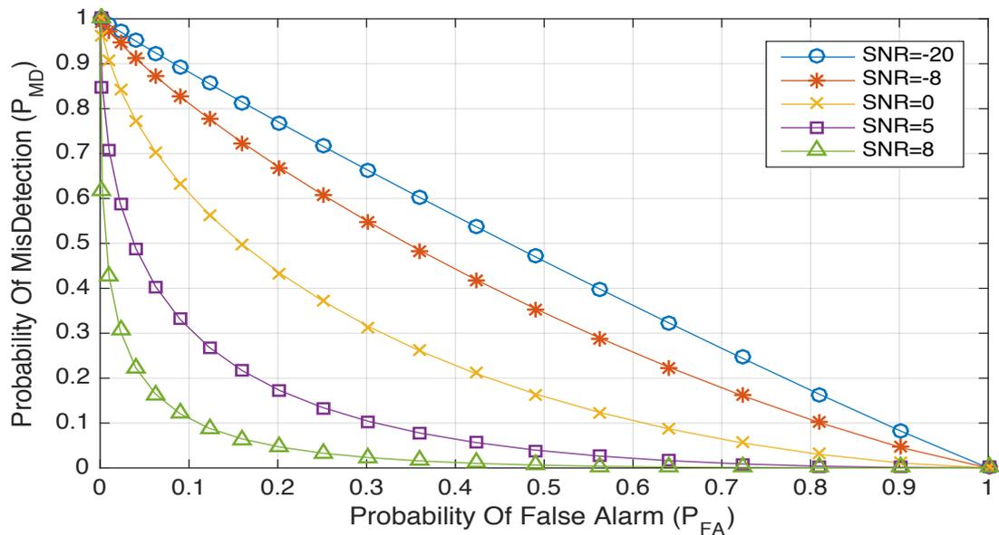
**Figure 3.13: Matched Filter Detection ROC curve for  $P_{MD}$  vs  $P_{FA}$ .**
