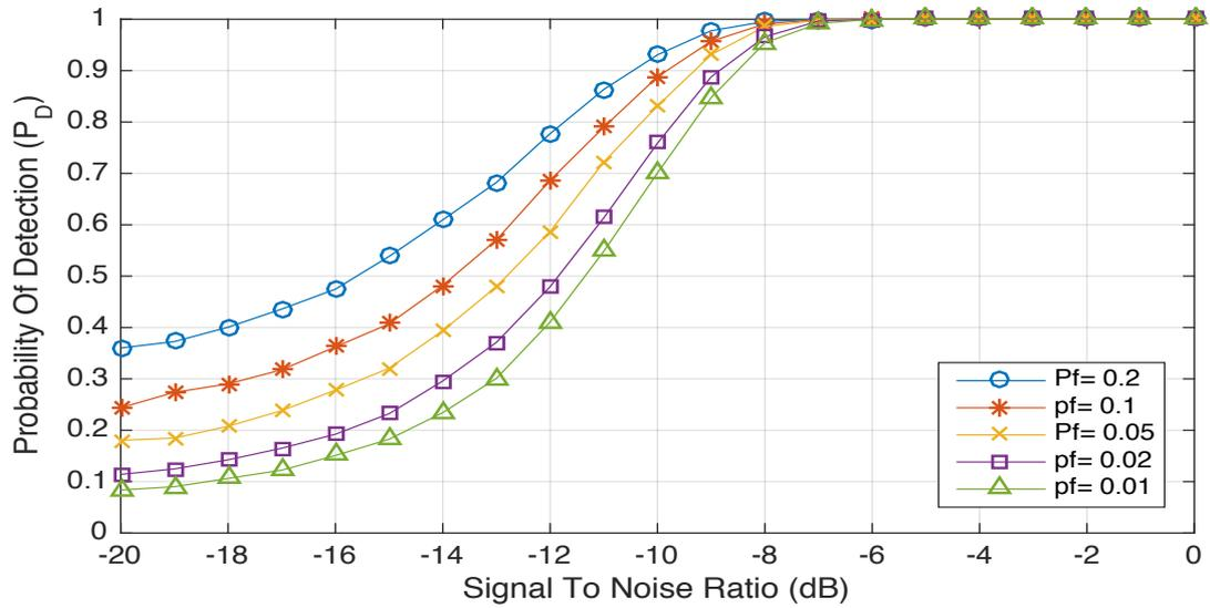
**Figure 3.8: Energy Detection ROC curve for  $P_D$  vs SNR with varying  $P_{FA}$ .**
