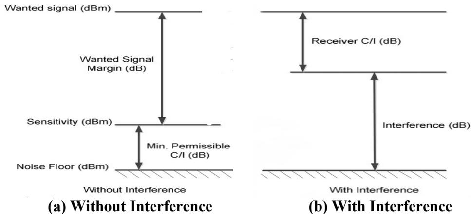
**Figure 2.3: Power levels used to determine presence/absence of interference**
