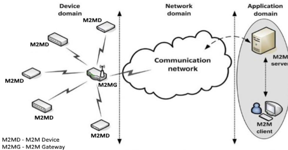
**Figure 2.14: Architecture of M2M Networks.**
