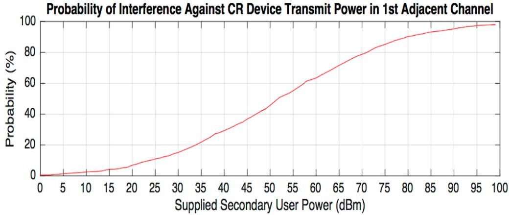
**Figure 3.5: Probability of interference against transmit power of 1<sup>st</sup> Adjacent SU.**
