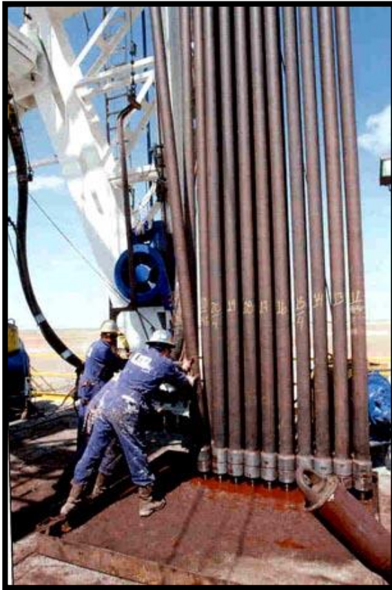
Plate 2.3: Drilling rig floormen setting back drill strands and exposed to ergonomic risk factors
