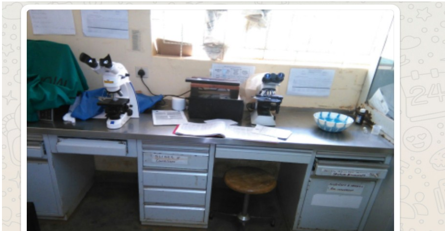
Plate 4. 3: Example of laboratory design that has provided a knee space under the work top
