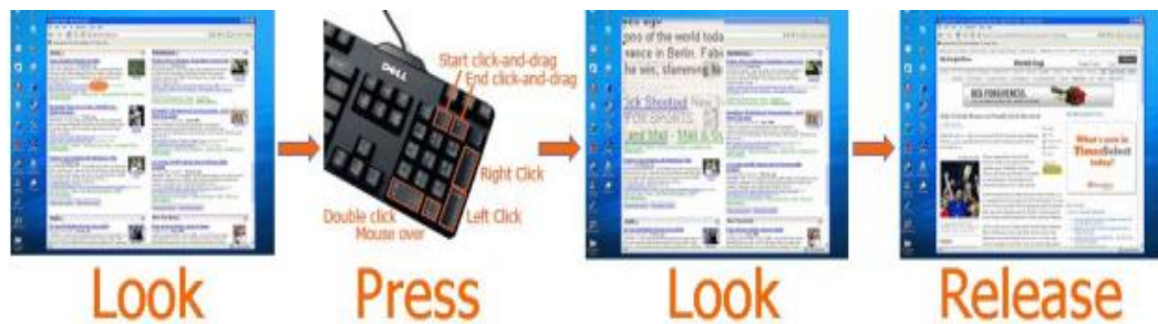
Figure 2.6: EyePoint technique for pointing and selection
