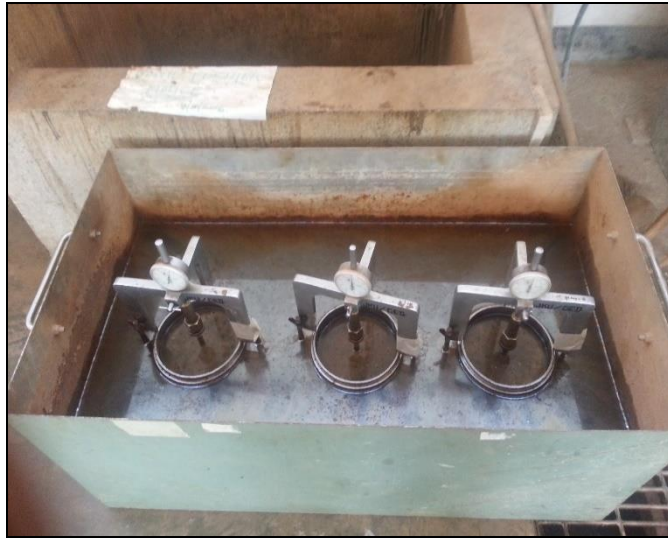
Plate 3.4: CBR specimens in soaking basin.
