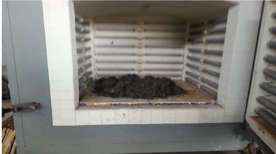
Plate 3.1: Heating kiln with soil sample in position
