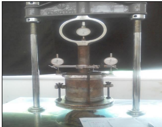
Plate 3.5: CBR test – specimen in position
