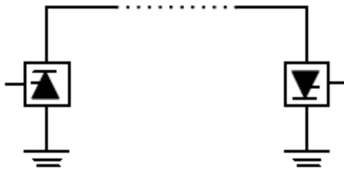
Figure 2.2: Monopolar HVDC Transmission system.
