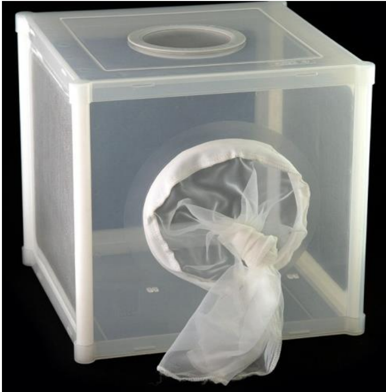
Fig.3.6 Cage 3. Locally made cage for the study (30x30x30cm) Courtesy of Seme Capentry Workshop, Eldoret, Kenya
