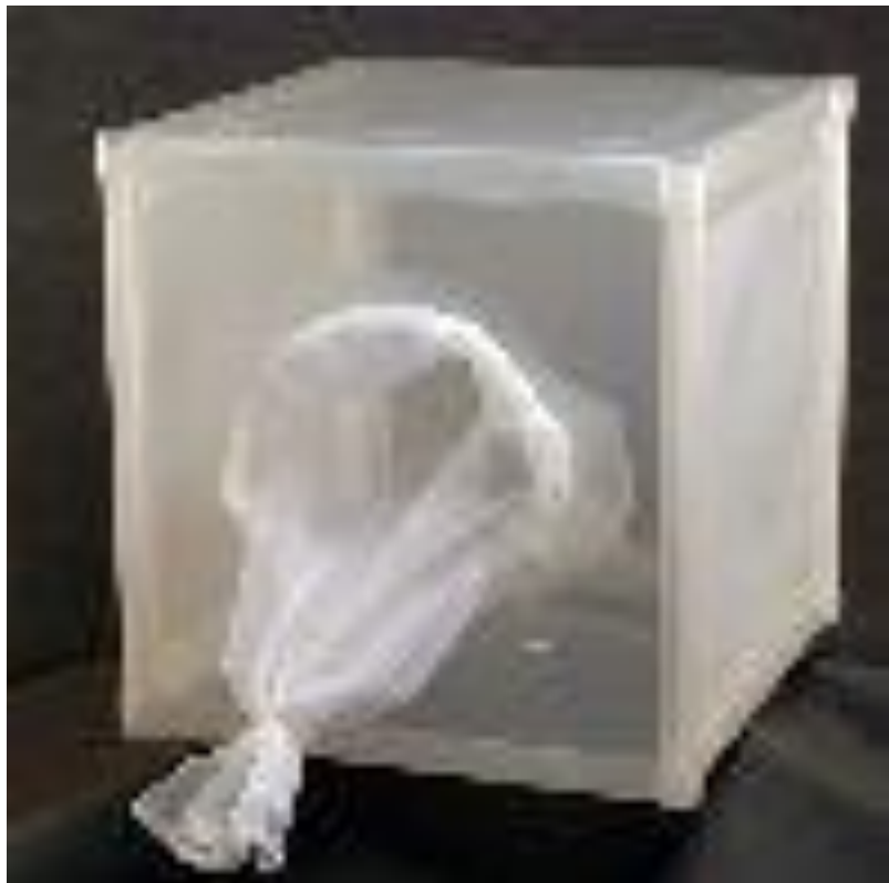
Fig 3.7. Cage 3. Locally made cage for the study (30x30x30cm) Courtesy of Seme Capentry Workshop, Eldoret, Kenya
