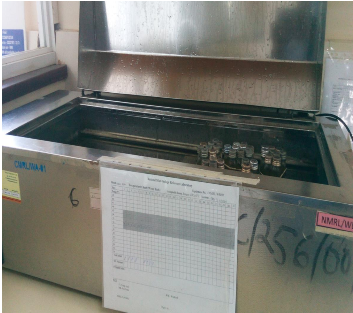
Incubation process at 44 degrees in a water bath for enumeration of coliforms
