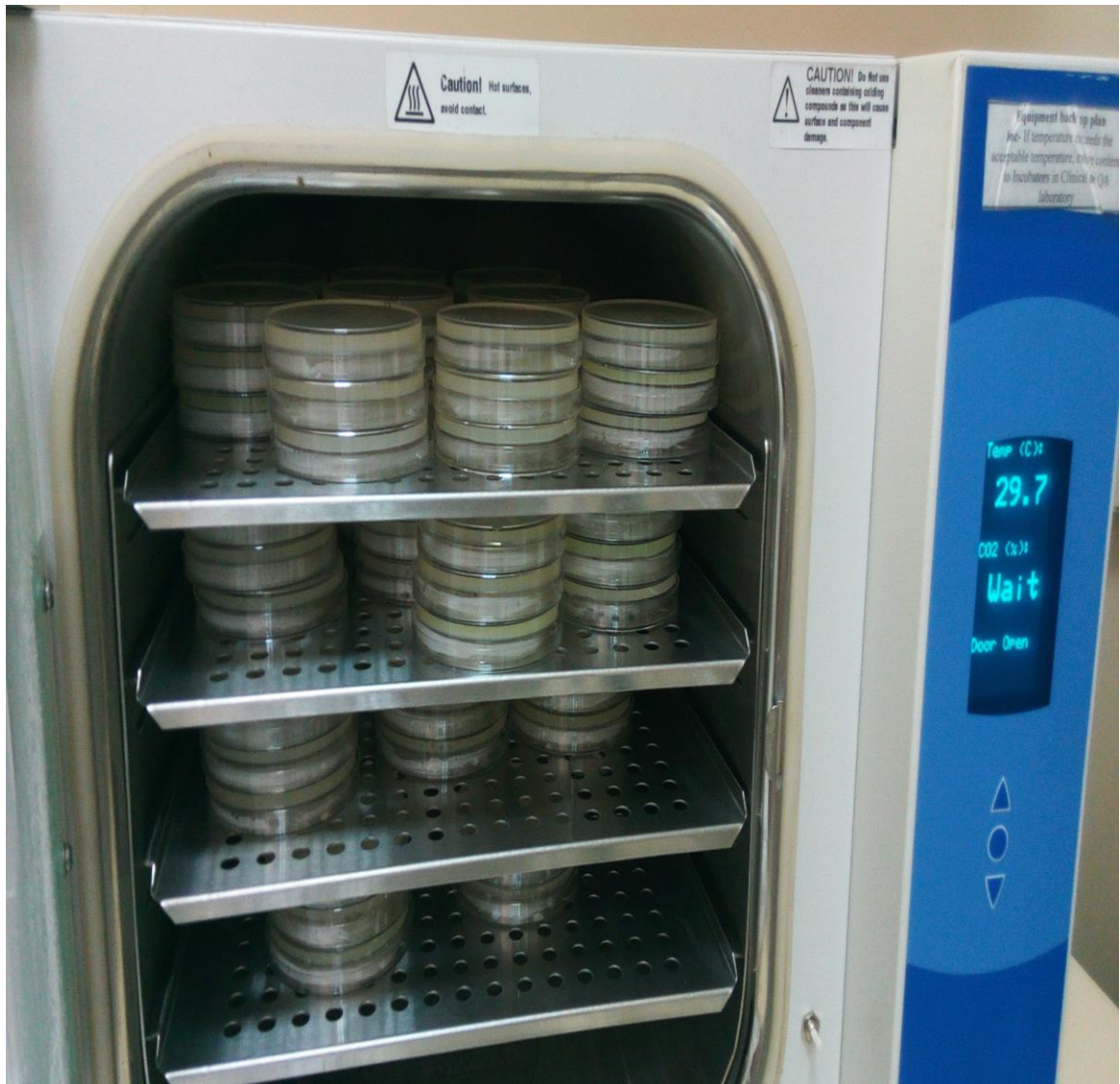
Incubation process at 30 degrees celcius for growth of microorganisms on plate count agar
