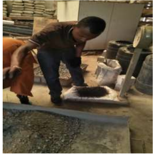
Fig.A-9-10. Adding RTSF in a mix
