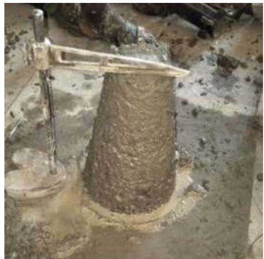
Fig.A-9-12. Slump test of RTSFRC mix
