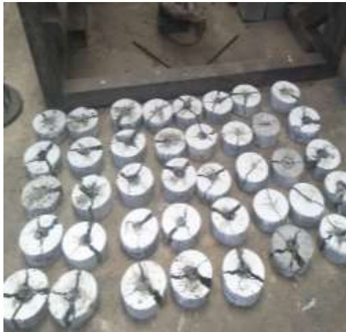
Fig.A-9-43. Ultimate failure mode of impact test specimens
