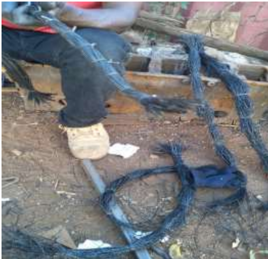
Fig.A-9-3. Arrangement of Recycled Steel tyre cords to be cut.
