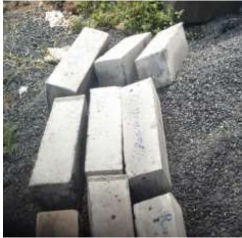
Fig.A-9-25. Drying of concrete beams to be tested
