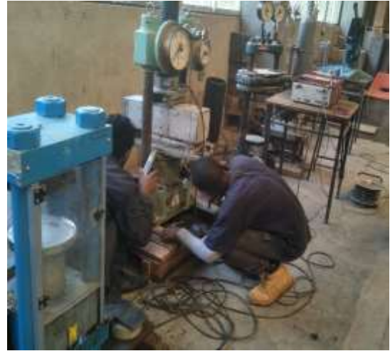
Fig.A-9-30. Installation of LVDTs
