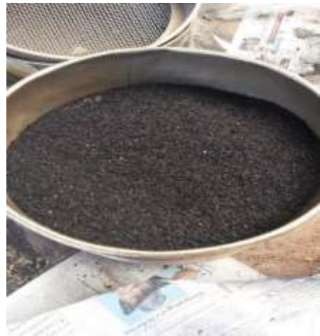
Fig.A-9-8. Sieving of Crumb rubber
