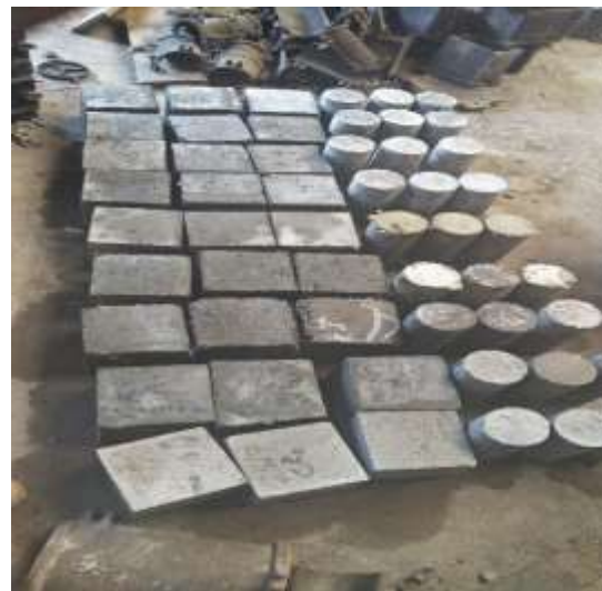
Fig.A-9-16. Concrete cubes and cylinders
