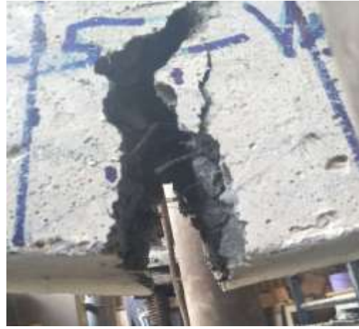
Fig.A-9-34. Flexural failure mode of RTSFRC
