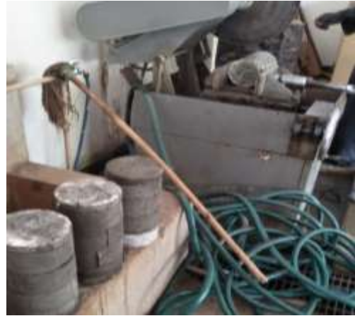
Fig.A-9-38. Cutting of Cylinders for impact test samples
