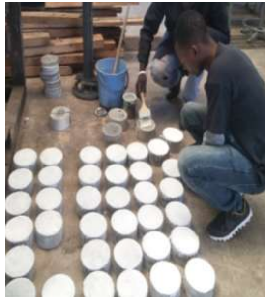
Fig.A-9-40. Smearing white paint on impact test specimens surface
