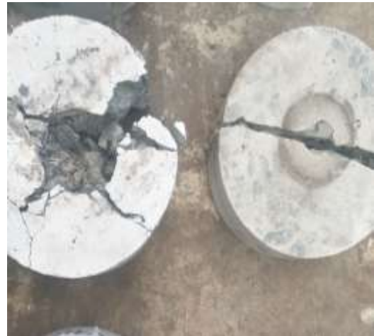
Fig.A-9-44. Ultimate failure mode of RTSFRC vs Plain mix
