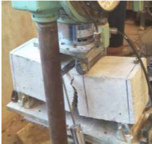
Fig.A-9-29. Flexural test of the beam
