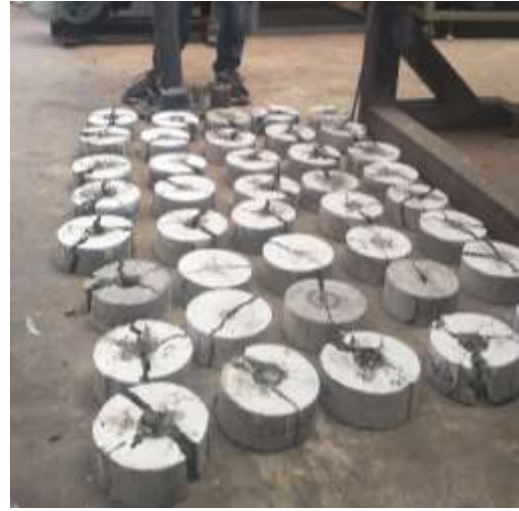
Fig.A-9-42. Ultimate failure mode of impact test specimens
