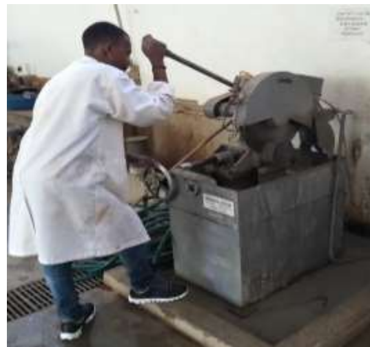
Fig.A-9-36. Cutting of Cylinders for impact test samples
