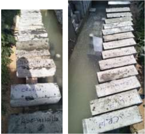
Fig.A-9-26. Placing Concrete beams in curing tank
