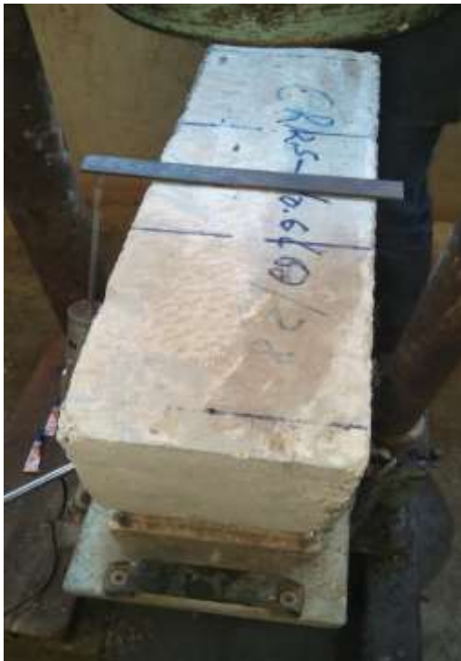
Fig.A-9-28. Arrangement of beam sample for flexural strength test
