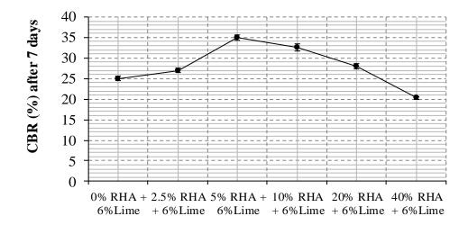
Figure 4.5: Effect of RHA on the bearing capacity of expansive clay soils for 6% NL
