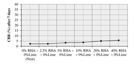
Figure 4.2: Effect of RHA on the bearing capacity of expansive clay soils for 0%
