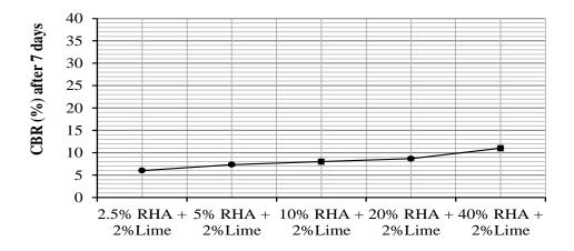
Figure 4.3: Effect of RHA on the bearing capacity of expansive clay soils for 2% NL
