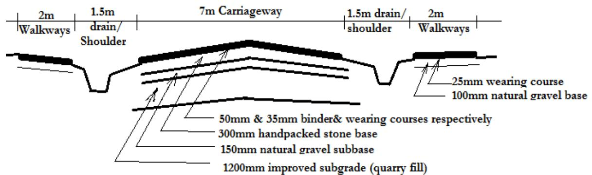
**Figure 4.11: Typical road cross section for Enterprise road**
