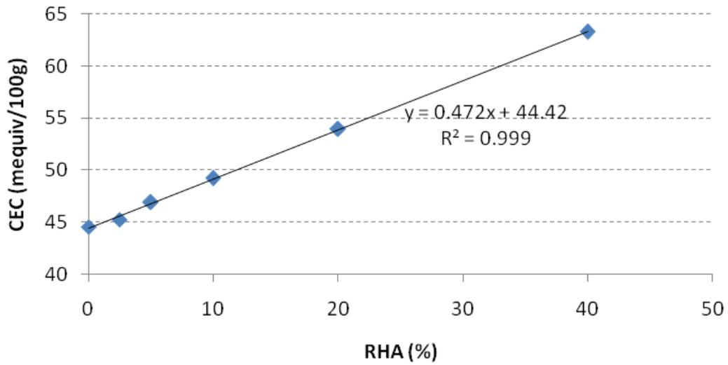
**Figure 4.9: Effect of RHA on the Cation Exchange Capacity of Soil Treated 2% NL**
