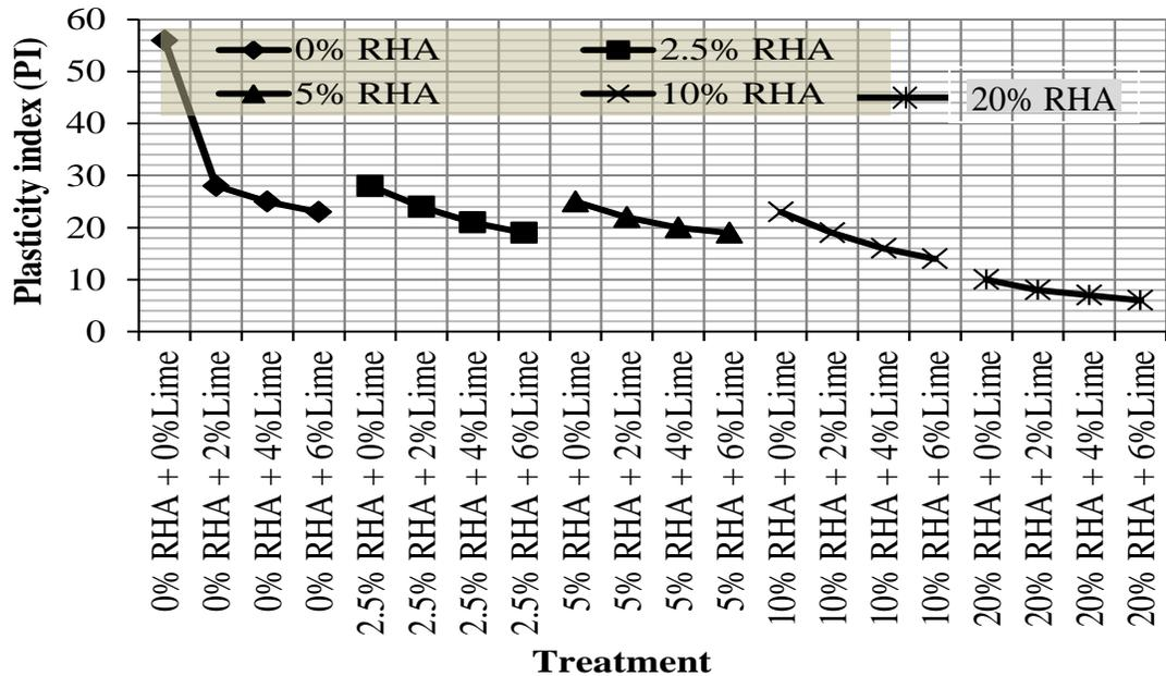
**Figure 4.8: Effect of RHA and NL on Plasticity**
