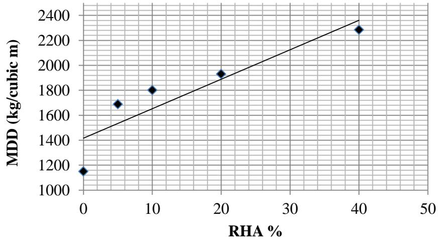
**Figure 4.1: Effect of Rice Husk Ash on the density of subgrade material**
