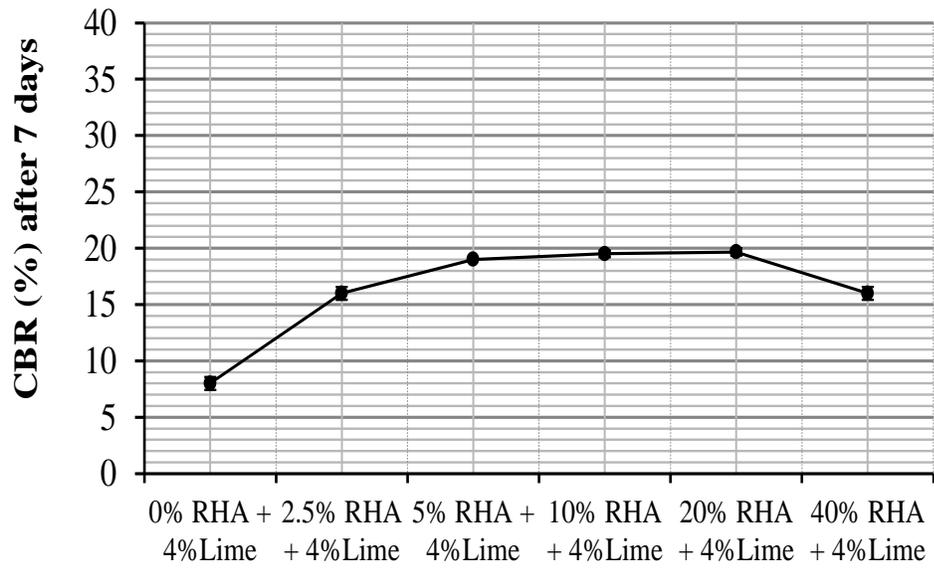
**Figure 4-4: Effect of RHA on the bearing capacity of expansive clay soils for 4% NL**
