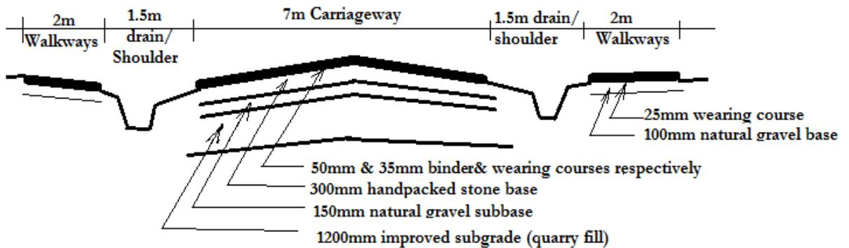
**Figure 4.11: Typical road cross section for Enterprise road**
