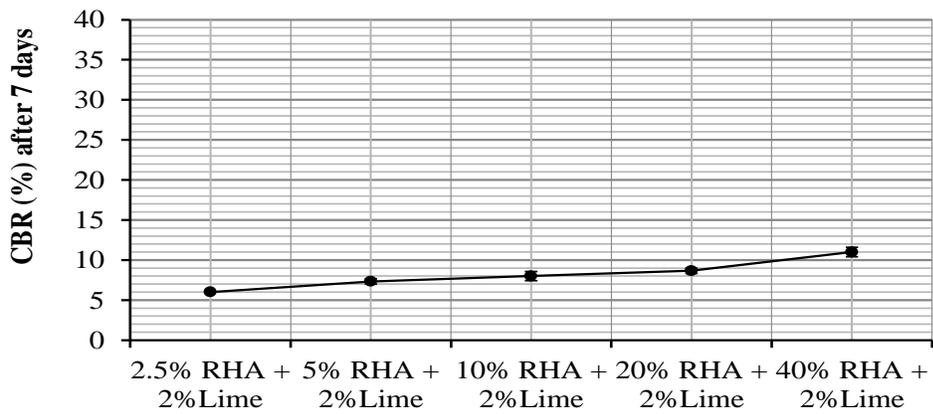
**Figure 4.3: Effect of RHA on the bearing capacity of expansive clay soils for 2% NL**
