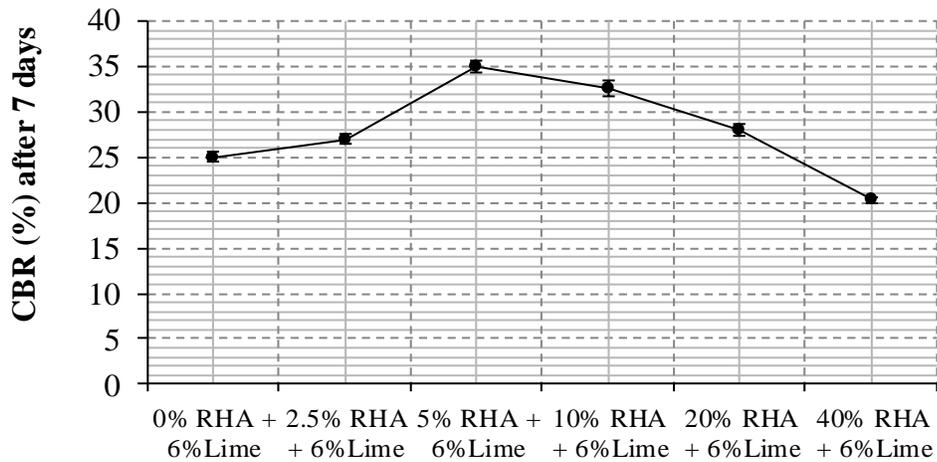
**Figure 4.5: Effect of RHA on the bearing capacity of expansive clay soils for 6% NL**
