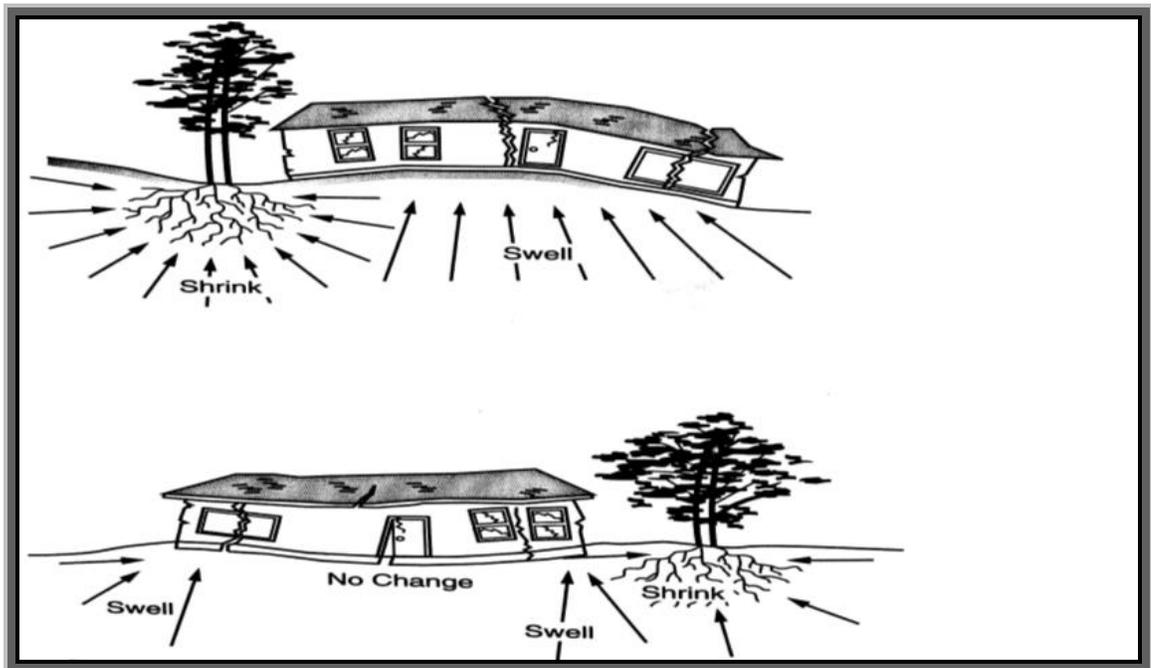
**Figure 2.1: Effects of swelling and shrinking behavior of expansive clay soils on structures** (Source: Bell and Howell, 1981)
