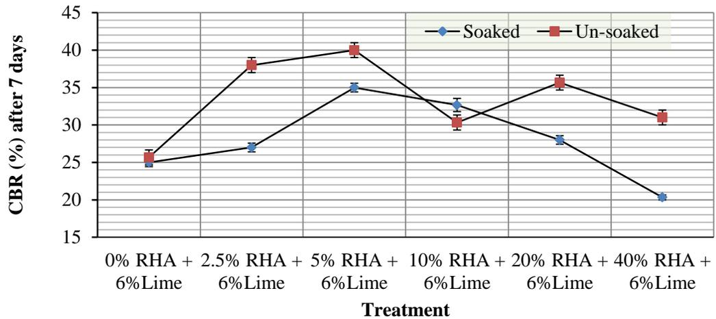
**Figure 4.6: Effect of soaking on subbase strength**
