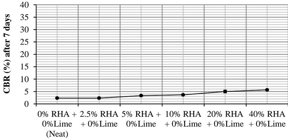
**Figure 4.2: Effect of RHA on the bearing capacity of expansive clay soils for 0% lime**
