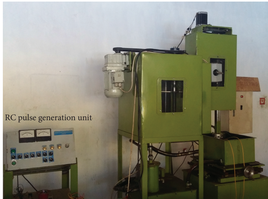
Figure 3.1: EDM machine based on RC pulse generation
