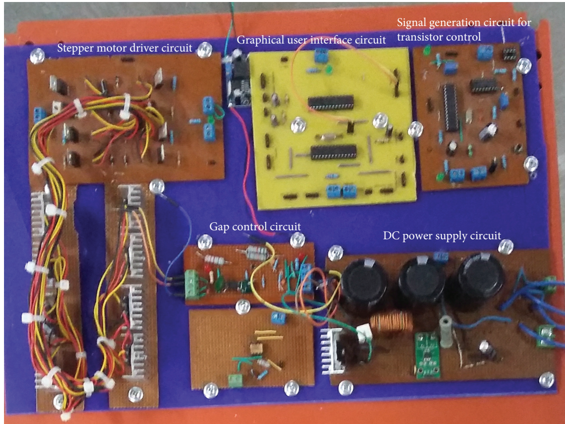
Figure 3.2: EDM control and pulse generation circuit based on Arduino Atmega 328P microprocessor
