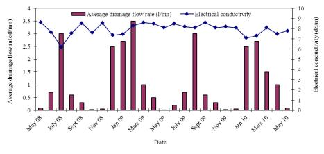
Figure 9. Observed values of drainage flow rate and electrical conductivity of drainage water.
