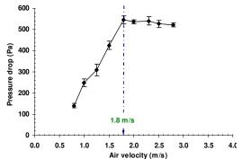
**Figure 1.** Fluidization characteristics of soybeans.
