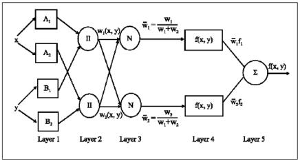
Figure 1. Schematic diagram of ANFIS model.
