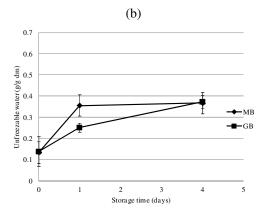
**Figure 4.** Evolution of freezable water (a) and unfreezable water (b) of Sangak bread baked on the metal bed (MB) and on gravel bed (GB) during storage at 20°C (data are the average of 3 baking temperatures).
