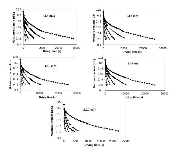
**Figure 4.** Drying curves of paddy at different air temperatures  $[(\bullet) 30^{\circ}\text{C}, -40^{\circ}\text{C}; (\bullet) 50^{\circ}\text{C}; (\blacktriangle) 60^{\circ}\text{C}; (\times) 70^{\circ}\text{C}, and (\bullet) 80^{\circ}\text{C}]$  and air velocities.
