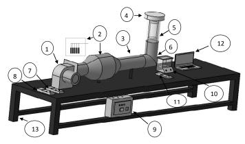
**Figure 1.** Schematic diagram of thin-layer dryer: (1) Fan and electrical motor; (2) Heating elements; (3) Duct and tunnel; (4) Chamber cap; (5) Drying chamber; (6) Mixing chamber; (7) Temperature and moisture meter; (8) Anemometer, (9) Thermostat and invertor; (10) Digital balance; (11) Input and output air temperature recorder; (12) Notebook, and (13) Chassis.
