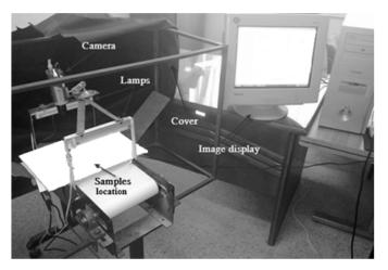
Figure 2. The machine vision system.
