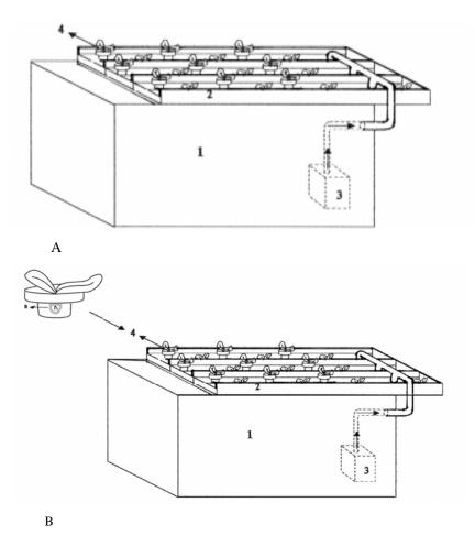
**Figure 1.** Schematic feature of the aquaponic system used for culture of fish and vegetables, 1. Fish tank, 2. Hydroponic troughs, 3. Water pump, 4. Lettuce cup, 5. A small cotton bag containing 10 g zeolite.
