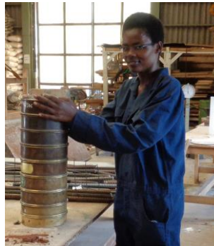
Plate 3-1 Particle size determination by sieve analysis
