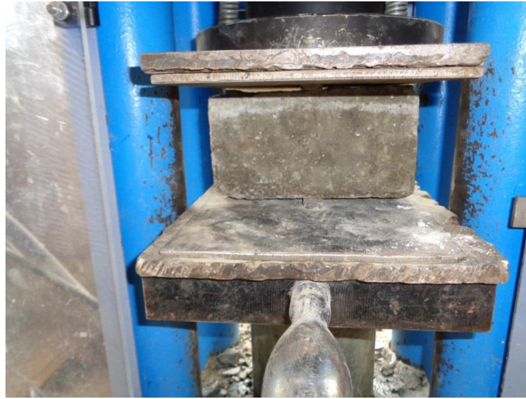
Plate 3-4 Set up for tensile strength test
