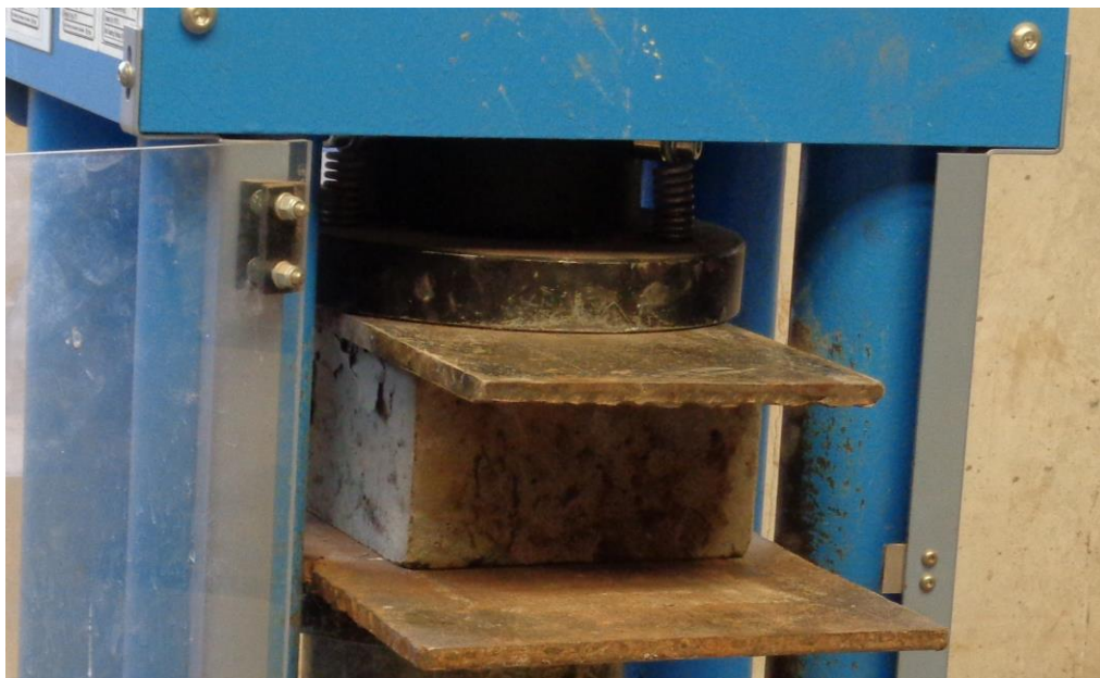
Plate 3-3 Set up for compressive strength test
