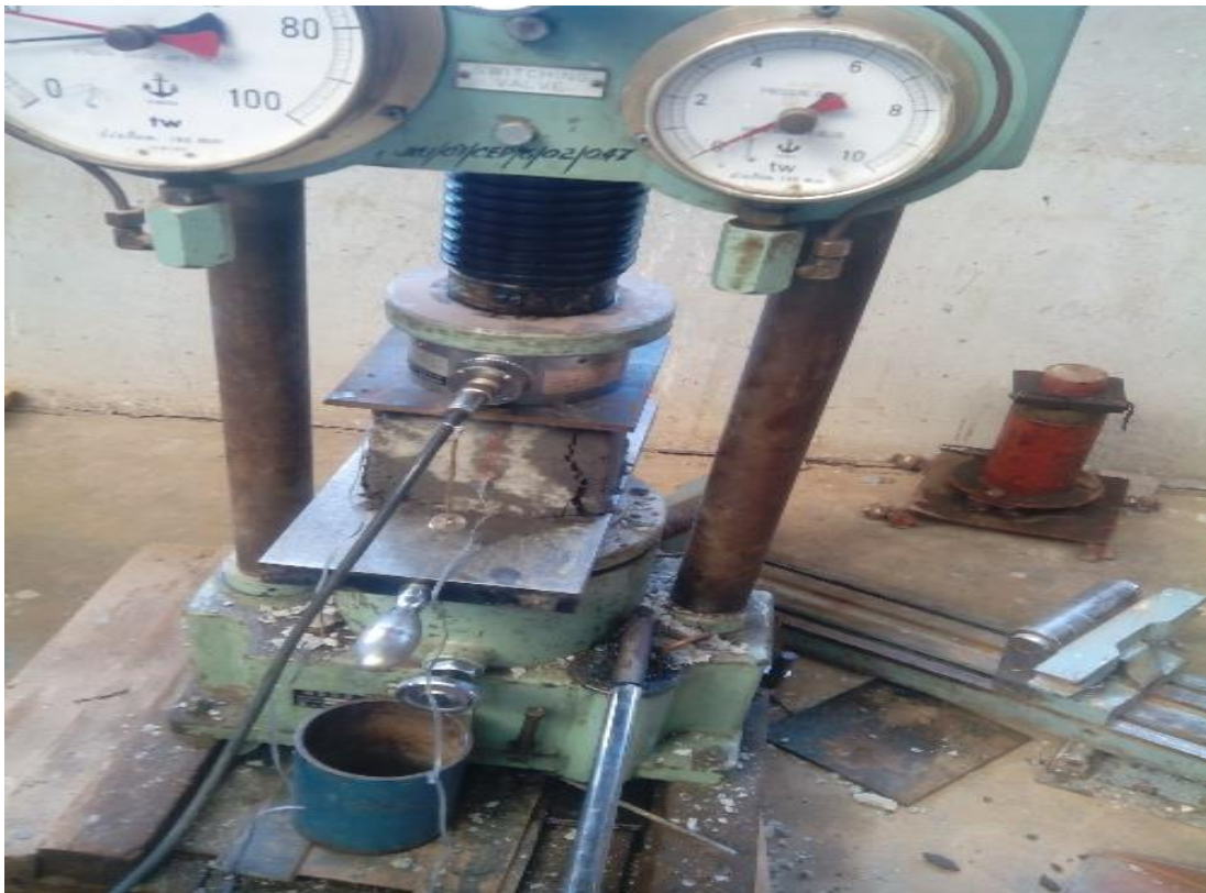
Plate 3.4: Cube crushing in progress
