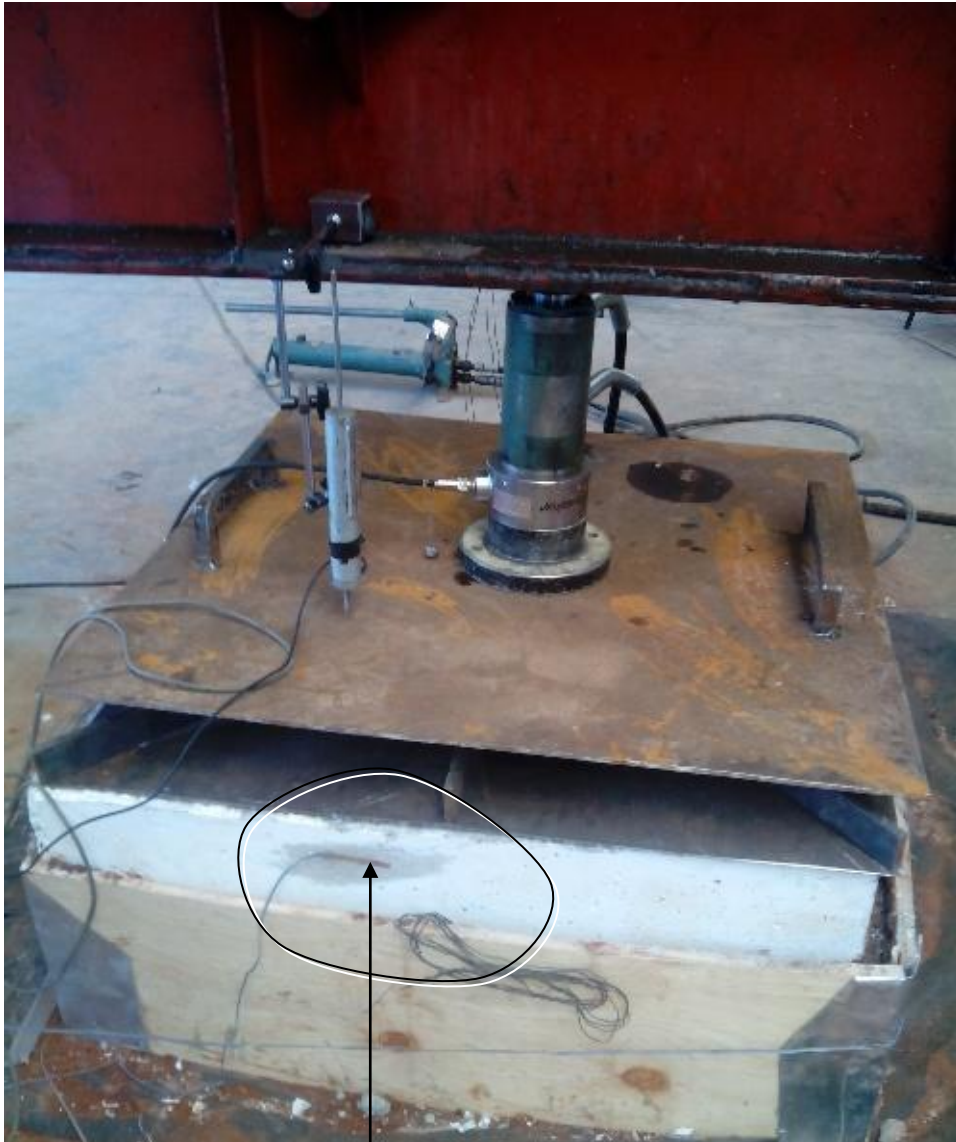
Strain gauge on all four sides of the concrete slab.
