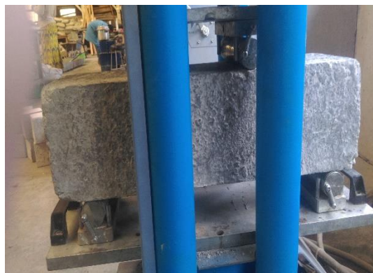
Figure 3.4: Flexural strength test
