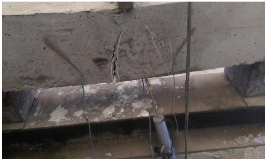
Figure 3.6: Sample beam testing for load versus deflection, shear stresses, flexural stresses and shear strains
