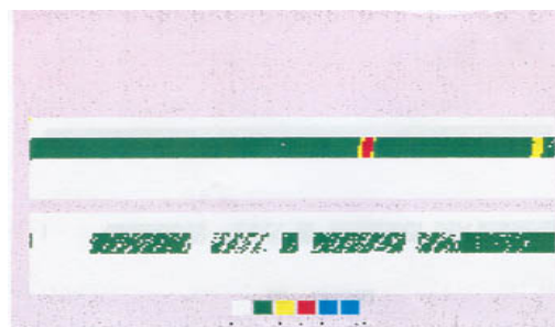
Figure 9. Colored band representing the intensity of applied load on the probe pressure cell.
