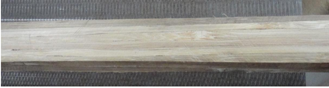
Plate 4.17 Proper bonding at the centre of Laminated panel
