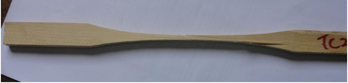
Plate 4.2 Tensile failure of a bamboo strip with outer skin removed
