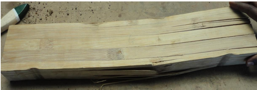
Plate 4.19 Mode of Failure in Laminated Bamboo Beam
