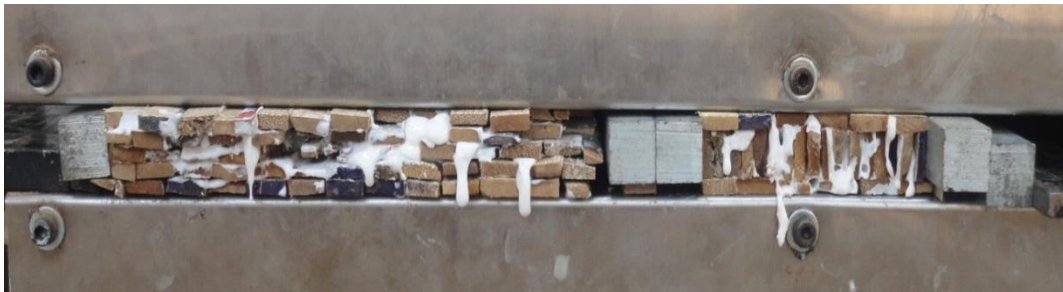
Plate 4. 15 Bleeding of glue under pressure
