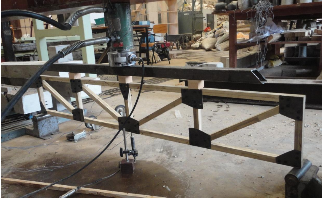
Plate 3.13 Truss Model Loading Setup
