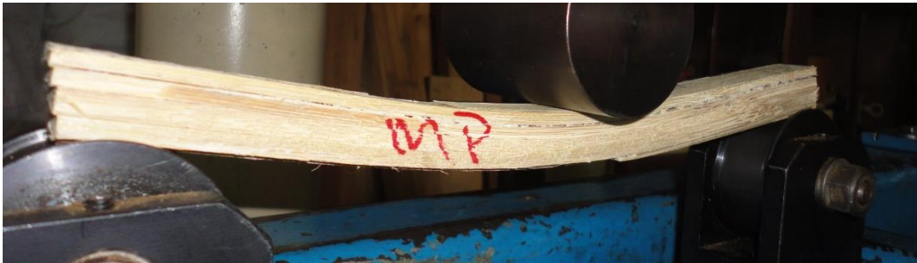
Plate 4.11 Beam specimen of Glue type 2
