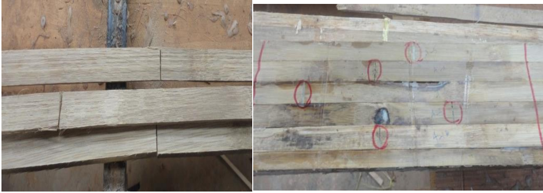
Plate 3. 8 Bamboo Panel Laminated with alternate joints
