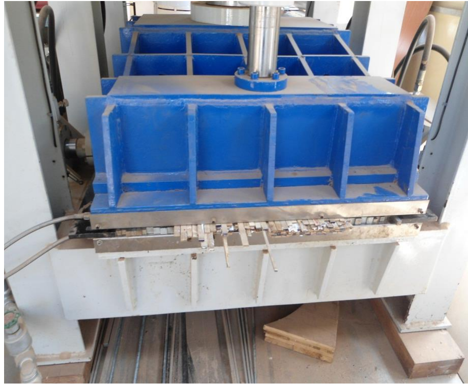
Plate 3.6 Cold Pressing Laminated Panel
