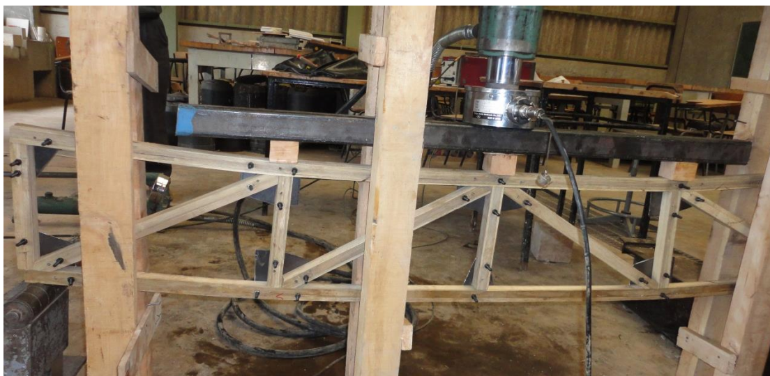
Plate 4.21 Deflected truss model under loading
