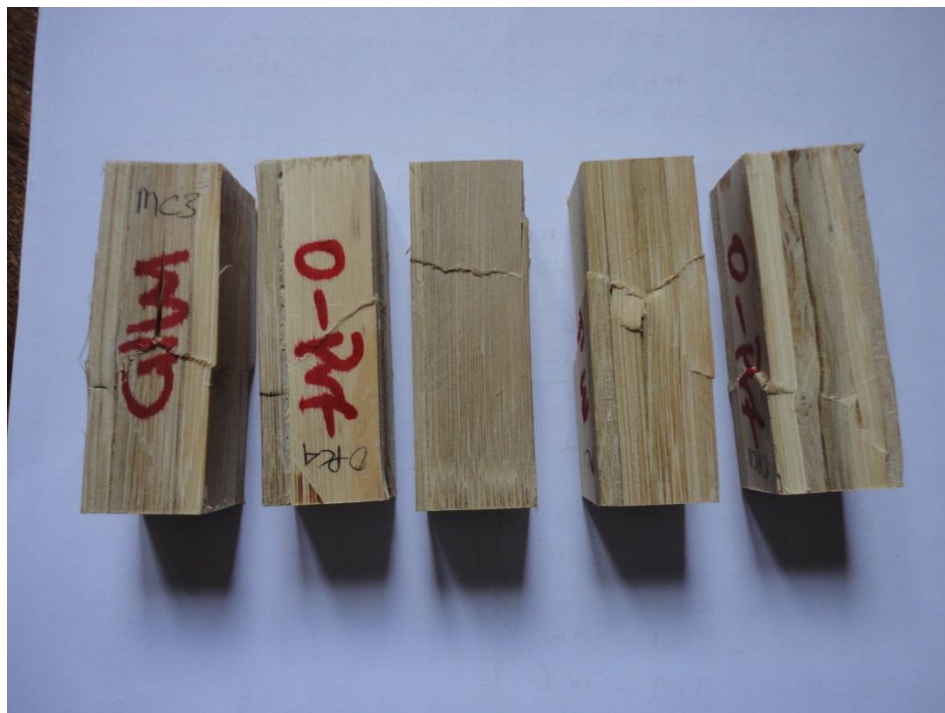
Plate 4.7 Failure mode under compression
