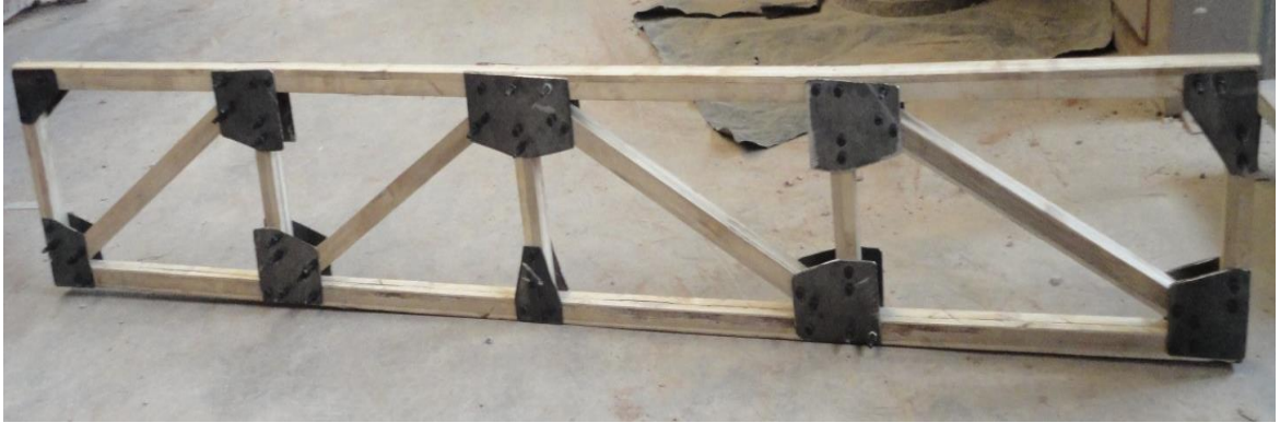
Plate 3.9 Glue Laminated Bamboo Beams Lattice Girder Truss Model
