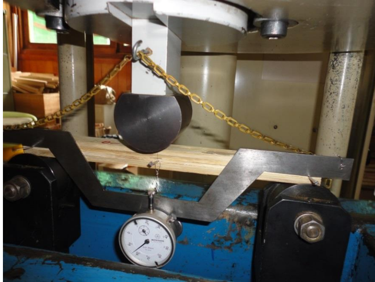
Plate 3.11 Static Bending Setup, Dial Gauge measures deflection
