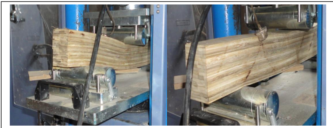
Plate 4.5 Beam under loading and after loading
