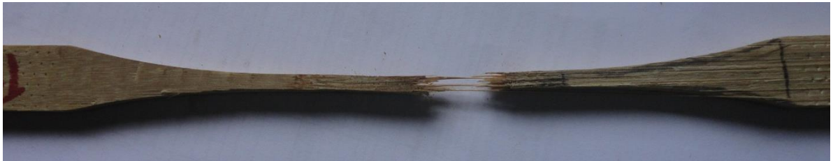
Plate 4. 1 Tensile failure of a bamboo strip with node at the center
