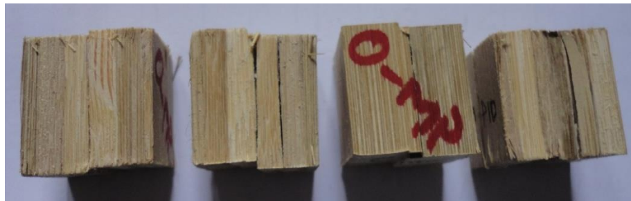
Plate 4.9 Specimens tested parallel to strips
