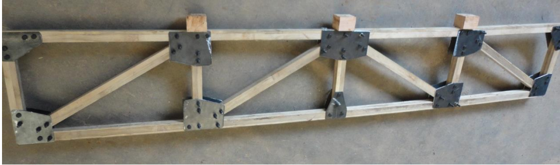
Plate 4.22 Truss model after testing
