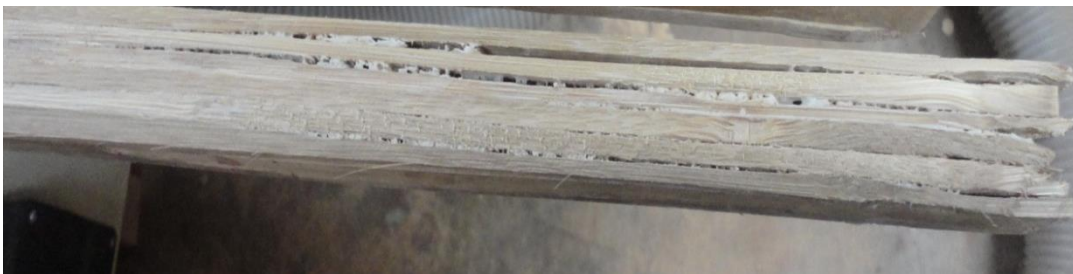
Plate 4.16 Voids on either ends of laminated panels
