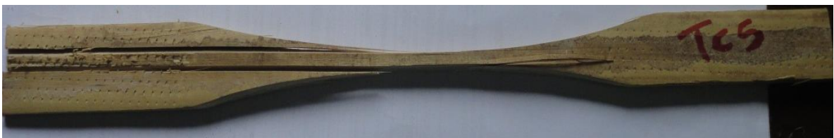
Plate 4.3 Tensile failure of a bamboo strip with outer skin intact and no node
