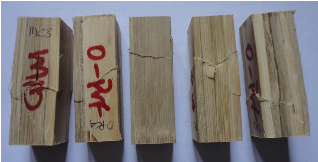
Plate 4.13 Specimens Failed by buckling – Glue Type 1
