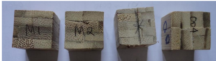
Plate 4.8 Specimens tested perpendicular to strips
