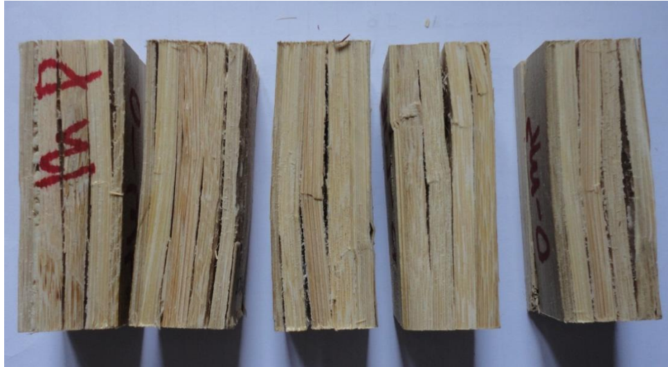
Plate 4.14 Specimens failed by delamination - Glue Type 2
