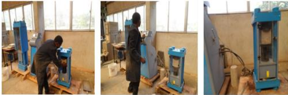
Figure 3.2.2: Compressive strength test
