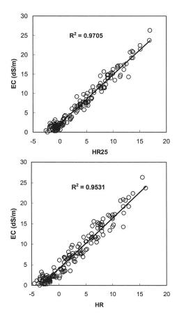
**Figure 2.** The relationship between the measured Electrical Conductivity (EC) and the Hydrometer readings corrected for 25°C (HR25) and uncorrected (HR) of the irrigation waters in Yazd Province, Iran.
