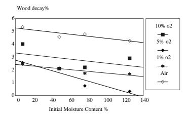
**Figure 3.** Regression between moisture content and wood decay by *C. versicolor* at 1, 5, 10, and 21 % oxygen in Scots pine.
