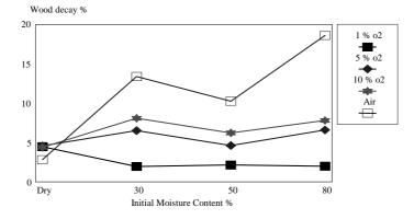
**Figure 10.** Relationship between moisture content and wood decay. at several levels of oxygen by *C. globosum* in beech.
