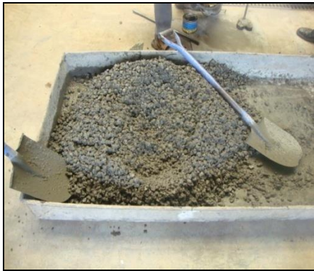
Plate 3.2: Wet concrete ready for testing
