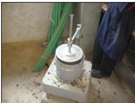
Plate 3.3: Vee-Bee consistometer test
