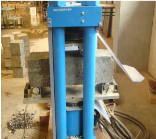
Plate 3.9: Experimental set-up for flexural strength test
