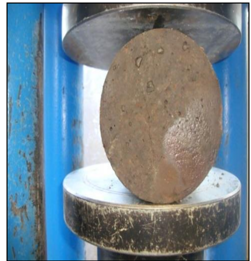
Plate 3.8: Crack pattern at failure
