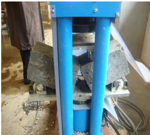
Plate 3.10: Crack pattern at failure
