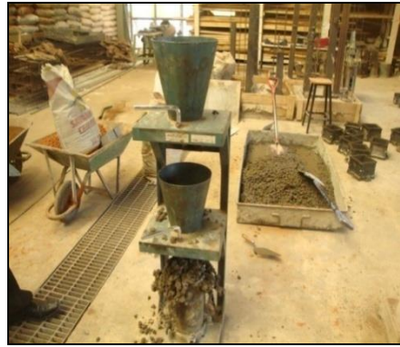
Plate 3.4: Compacting Factor Test
