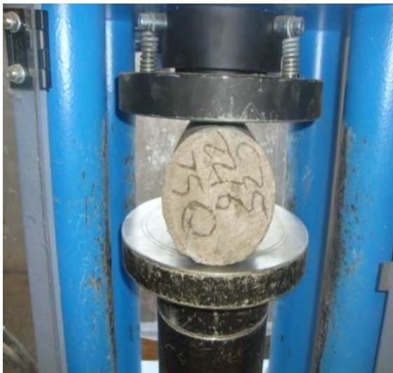
Plate 3.7: Experimental set-up for split tensile test
