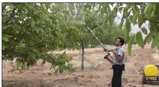
Figure 5. Designed and fabricated telescoping sprayer in operation.
