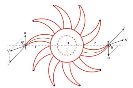
Figure 9. LERN with various velocity components while in operation.
