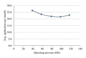
**Figure 7.** Average application rate of LERN at varying operating pressures.
