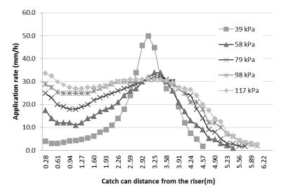
Figure 4. Radial water distribution pattern of LERN at varying operating pressures.
