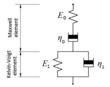
**Figure 1.** Diagram of the four-element Burgers Model composed of Maxwell and Kelvin–Voigt elements in series.
