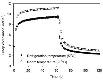
**Figure 3.** Creep compliance curves of frankfurter samples analyzed at refrigeration and room temperature during compression and recovery phases. The bars indicate standard errors.
