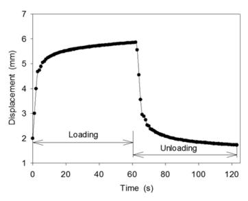
Figure 2. Creep behavior of a frankfurter sample analyzed at refrigeration temperature.
