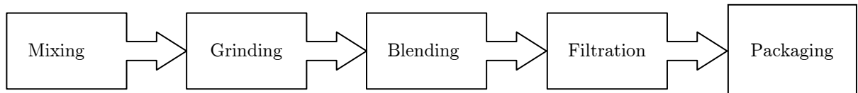
Figure 0.1: Steps in the paint manufacturing process
