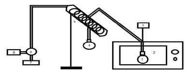
**Figure 2.** The schematic diagram of microwave vacuum, (1) Airtight jar; (2) Microwave heating chamber; (3) Thermometer; (4) Collectors jar; (5) Condenser; (6) Vacuum pump; (7) Pressure controller; (8) Vacuum control valve.
