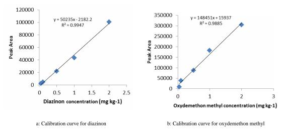
**Figure 2**. Calibration curve for (a) Diazinon, and (b) Oxydemethon methyl.
