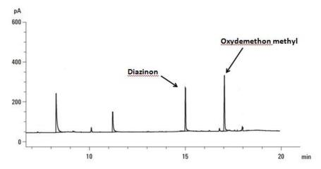
**Figure 1.** Representative chromatogram (GC/NPD) of diazinon and oxydemethon methyl standard spiked in blank tomato matrix.
