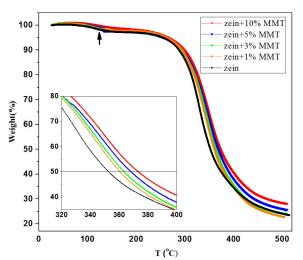
**Figure 4.** TGA curves of zein-MMT nanocomposite films prepared using a high power ultrasonic probe. The arrow shows the weight loss of low molecular weight compounds. Inset shows an enlarged part of the curves from 320 to 400°C.
