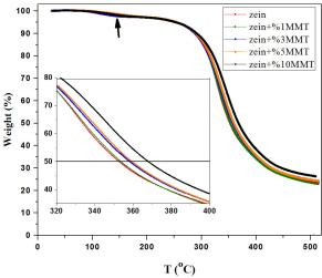
**Figure 3.** TGA curves of zein-MMT microcomposite films prepared using an ultrasonic bath. The arrow shows the weight loss of low molecular weight compounds. Inset shows an enlarged part of the curves from 320 to 400°C.
