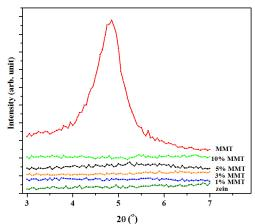
**Figure 2**. XRD patterns of MMT, zein film and nanocomposites of zein-MMT prepared using a high power ultrasonic probe.
