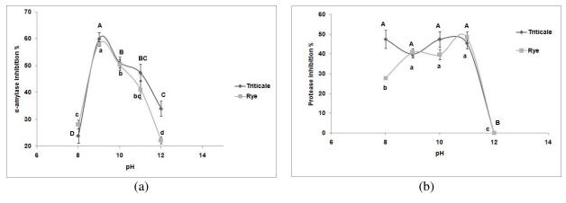
**Figure 3.** The effect of pH on inhibition of potato tuberworm  $\alpha$ -amylase (a) and protease (b) by extracts from triticale and rye. Means followed by the same letters are not significantly different by Tukey's test (P< 0.05).
