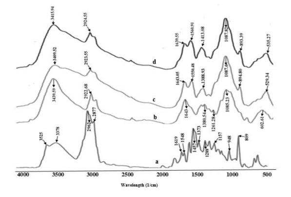
**Figure 1.** FTIR spectra of: (a) Thyme essential oil; (b) Chitosan powder; (c) Chitosan nanoparticle, and (d) Thyme oil loaded chitosan nanoparticle with chitosan: Thyme essential oil weight ratio of 1:0.4.
