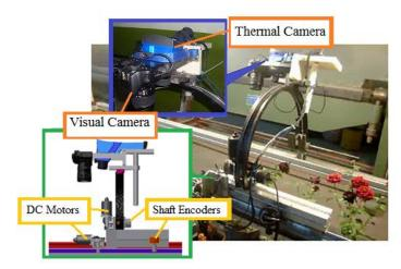
Figure 1. The developed automatic image capturing set-up.
