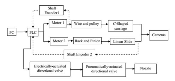
Figure 3. Block diagram of the machine vision and smart spraying system.
