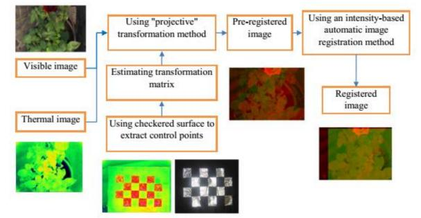
Figure 6. The registration procedure of the thermal and visible images.
