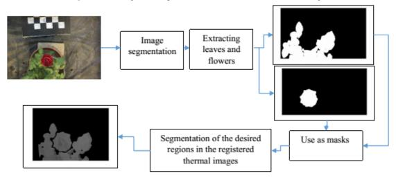
Figure 7. Segmentation algorithm for the thermal images.
