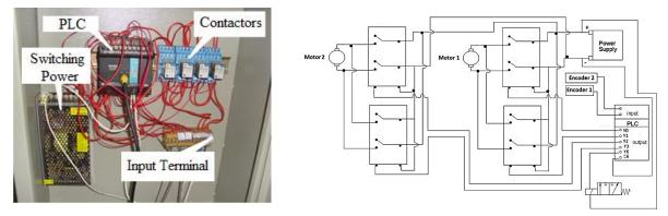
Figure 4. Electrical control circuit of the system.
