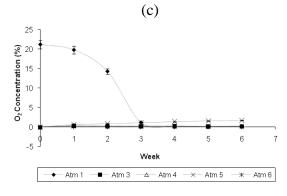
**Figure 1.** Evolution of  $N_2$  (a),  $CO_2$  (b) and  $O_2$  (c) concentrations in the packages : Atm 1: Air; Atm 3: 40%  $CO_2/60\%$   $N_2$ ; Atm 4: 60 %  $CO_2/40\%$   $N_2$ ; Atm 5: 100%  $CO_2$ , Atm 6: 100%  $N_2$ .
