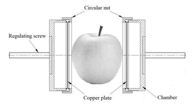
Figure 2. The schematics of the probes.
