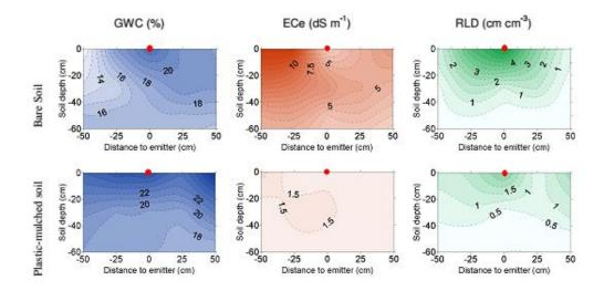
**Figure 4.** Gravimetric soil Water Content (GWC), soil salinity (ECe) and Root Length Density (RLD) contour lines of the bare and plastic-mulched soil treatments delineated for the 0-60 cm soil depth under the irrigation lateral. The soil samples were taken at three soil depths (0-20, 20-40 and 40-60 cm) in five points located at 25 cm increments along a 1-m segment of the lateral with the emitter (red dot) positioned in the center.
