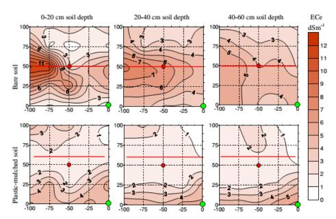
**Figure 2.** Soil salinity (ECe): Contour maps of ECe measured in the wetted area of the emitter in bare and plastic-mulched soil treatments insoil samples taken at 0-20, 20-40 and 40-60 cm soil depths on a  $25\times25$  cm grid of a 1 m<sup>2</sup> square area with the emitter (red dot) located in the center (X=-50 cm, Y= 50 cm) and the nectarine tree trunk (green dot) located in a corner of the area (X= 0 cm, Y= 0 cm). The horizontal red line represents the irrigation lateral.
