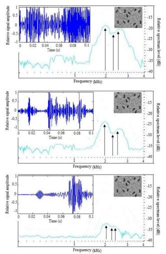
Figure 6. The acoustic frequency of *Triboium confusum* inside a wheat grain mass having several larvae and adult insects (from top to bottom: distance of 10, 20 and 30 cm, respectively).
