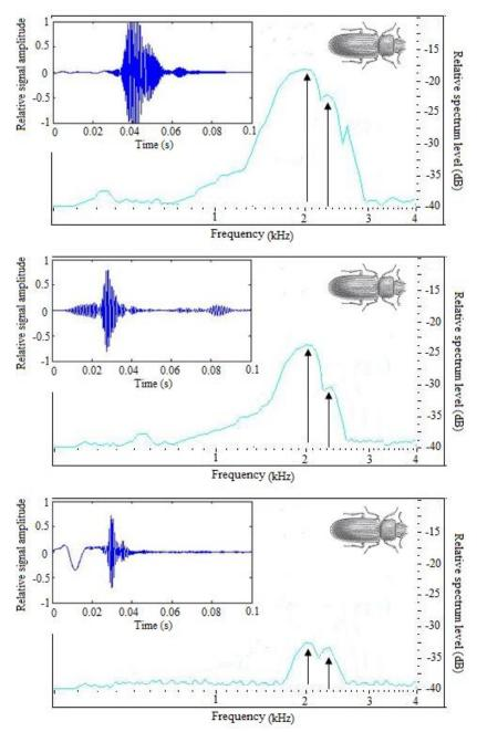
Figure 5. The acoustic characteristics of the adult insect of *Triboium confusum* recorded within wheat grain mass at different distances of insect and audio sensor (from top to bottom 10, 20 and 30 cm, respectively).
