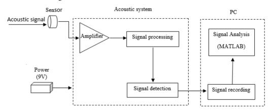
Figure 1. Flow diagram for acoustic signal detection and signal analysis of insect pests within a grain bulk.
