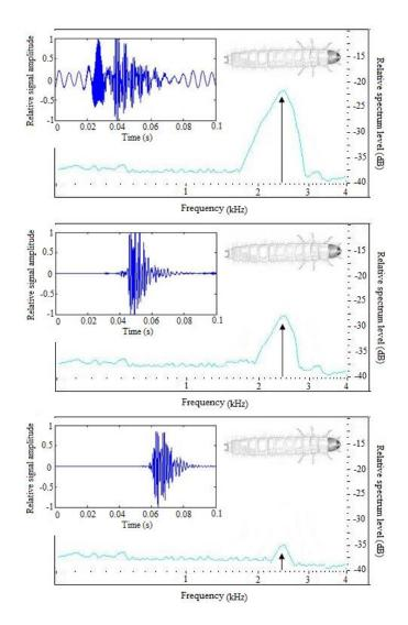
Figure 4. The acoustic characteristics of *Triboium confusum* in the larval stage, recorded within wheat grain mass at different distances of larvae and audio sensor (from top to bottom 10, 20 and 30 cm, respectively).
