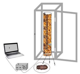
**Figure 2**. The soundproof test rig including: (1) PC; (2) Integrated signal detection and processing; (3) Acoustic insulation chamber; (4) Grain cylindrical graded repository; (5) Acoustic sensor; (60 *Triboium confusum*, (7) Thin grid.
