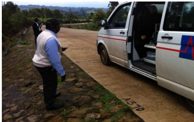
Figure 3.3: Slab Identity marking
