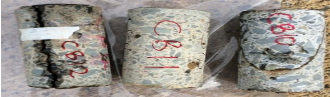
Figure 3.5: Extracted, cleaned and marked concrete cores
