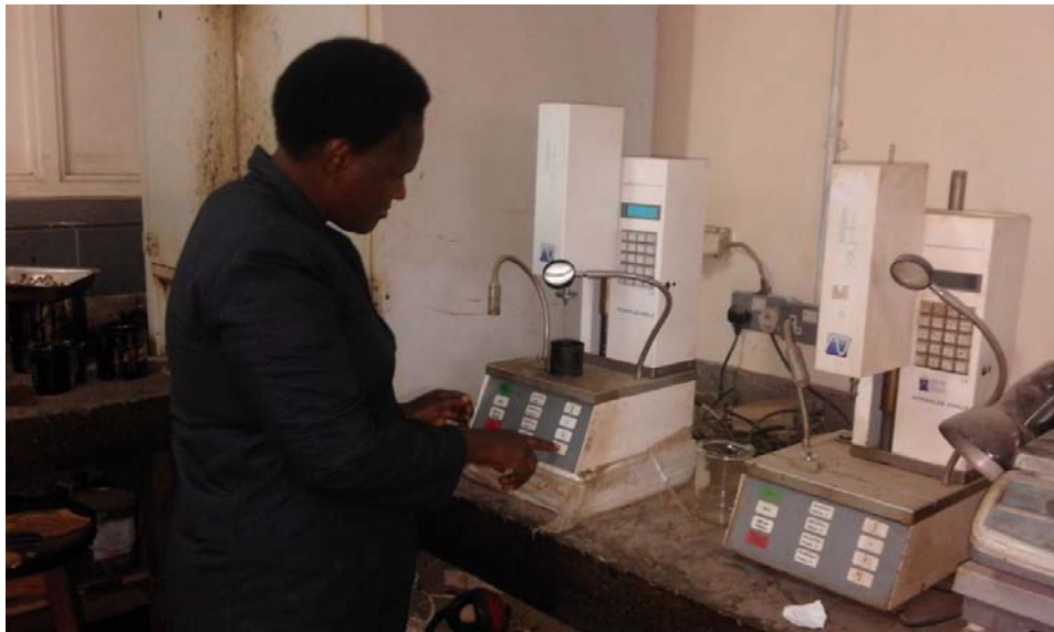
Plate 3:4. Penetration Testing Assembly
