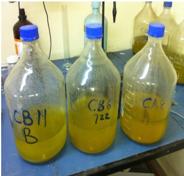
Figure 3.8: Solution used to determine the amount of cement in concrete
