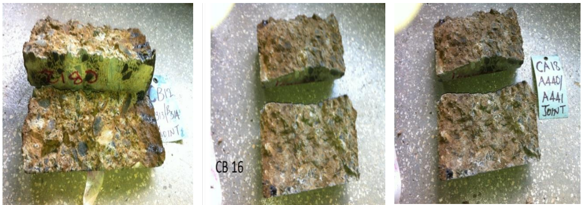
Figure 4.1: Full cracks development under saw-cut joints
