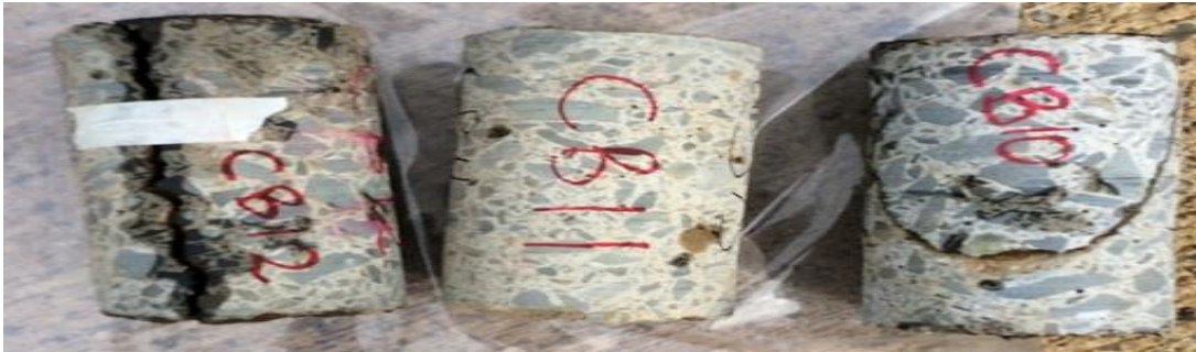
Figure 3.5: Extracted, cleaned and marked concrete cores
