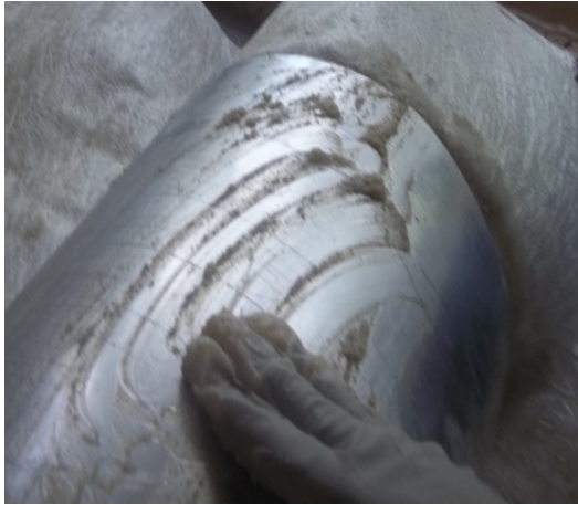
Plate 3.2: Application of Wax and other Associated Chemicals
