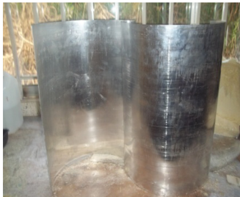
Plate 3.1: Folding of the Aluminium Sheet Metal
