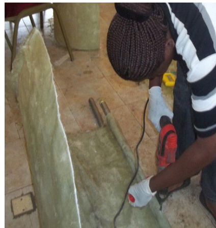
Plate 3.3: Laying of the Fibre Cloth, Trimming, Smoothing and Joining of the Blades.
