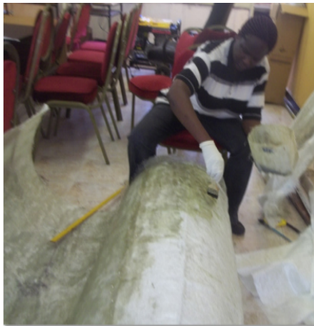
Plate 3.3: Laying of the Fibre Cloth, Trimming, Smoothing and Joining of the Blades.
