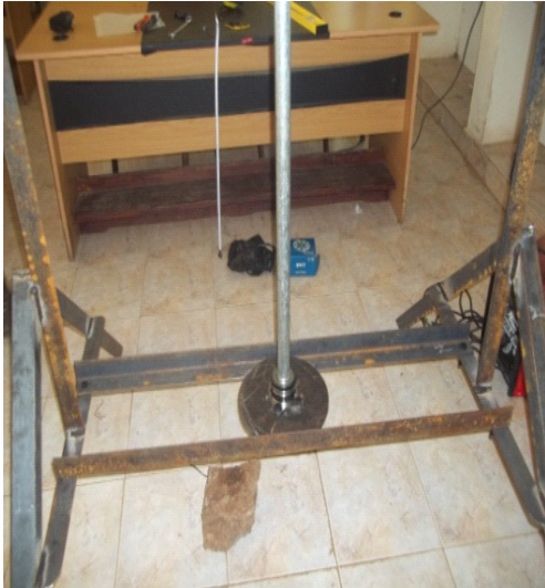
Live shaft and stand fabrication
