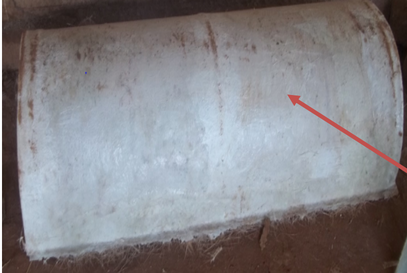
Plate 3.6: Application of releasing agent and gel on a Formica mould
