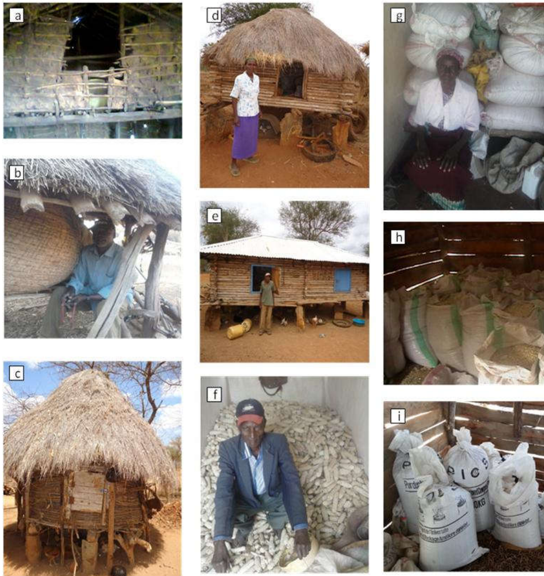
Figure 4.1: Maize storage structures across agro-ecological zones. a and b: traditional granaries; c: traditional crib; d: improved crib with grass thatch roof; e: improved crib with iron sheet roof; f: maize cobs stored on the floor in room; g: bagged maize grain stored in special room; h: bagged maize grain stored in crib; i: maize grain packed in plastic hermetic bags and stored in crib.
