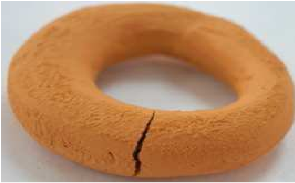
Figure 1: Effect of grain size on the strength of clay particles at 20 \mu\text{m} and temperature of 800°C after firing for five hours
