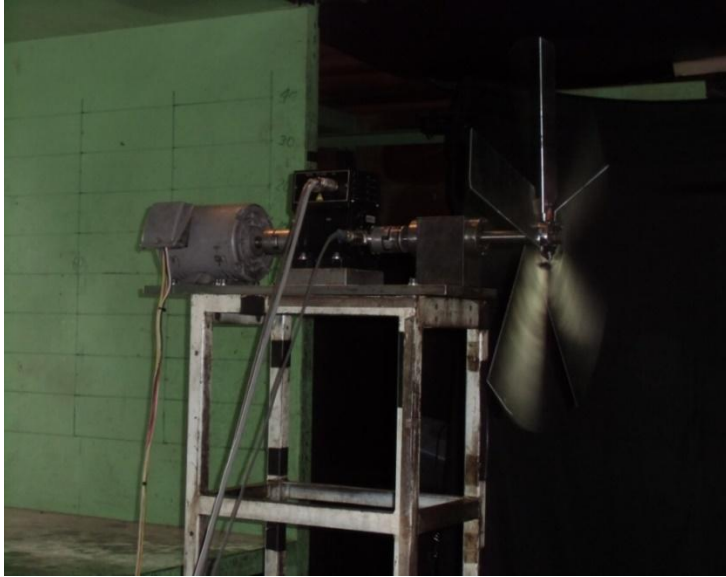
Figure 7: Turbine undergoing torque testing in the wind tunnel
