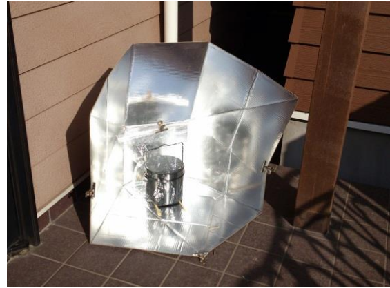
Fig. 2: Setting for high solar elevation
