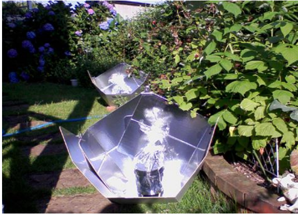
Fig. 1: Setting of Educooker003 for low solar elevation.
