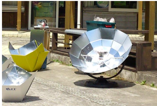
Fig. 15 Assembled concentrator type solar cooker
